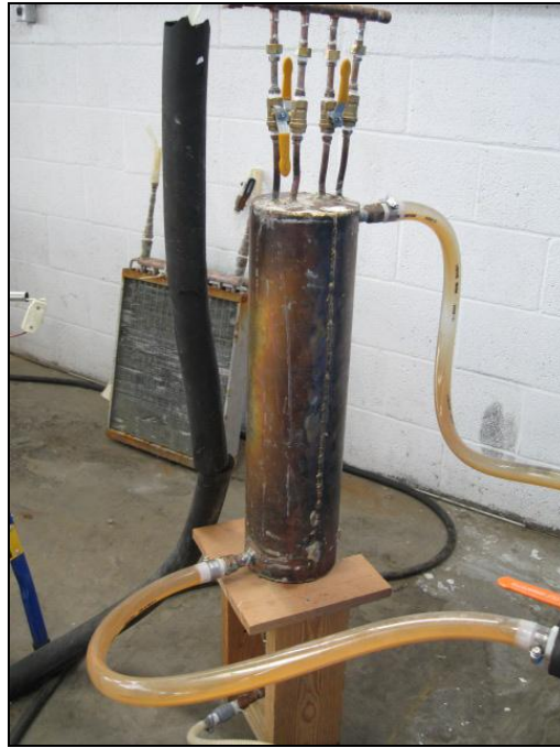
Figure 4: Helical coil heat exchanger without insulation [31]
