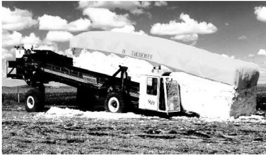
Figure 22 Australian module hauler loading a cotton module from the field
