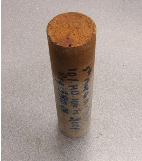
Figure 4.5 – The core shows significant iron deposit on the top as well as the sides
