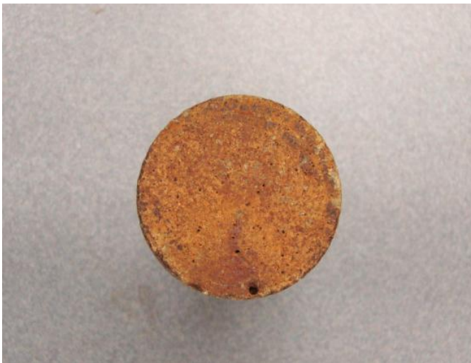
Figure 4.6 – Inlet face of the core shows the formation of wormhole
