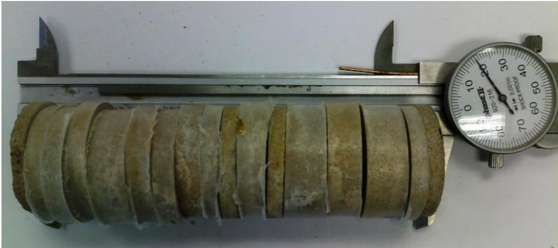
Figure 6.2 – Slices of Indiana Limestone core in which no GLDA was flowed stacked together and the length measured using a vernier caliper. The main scale of the vernier caliper shows 5 inches
