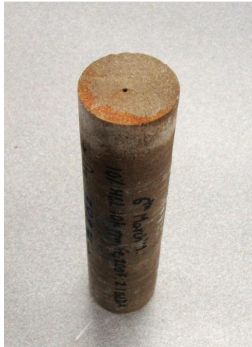
Figure 11.3 – This picture shows the deposit on the core face after the treatment
