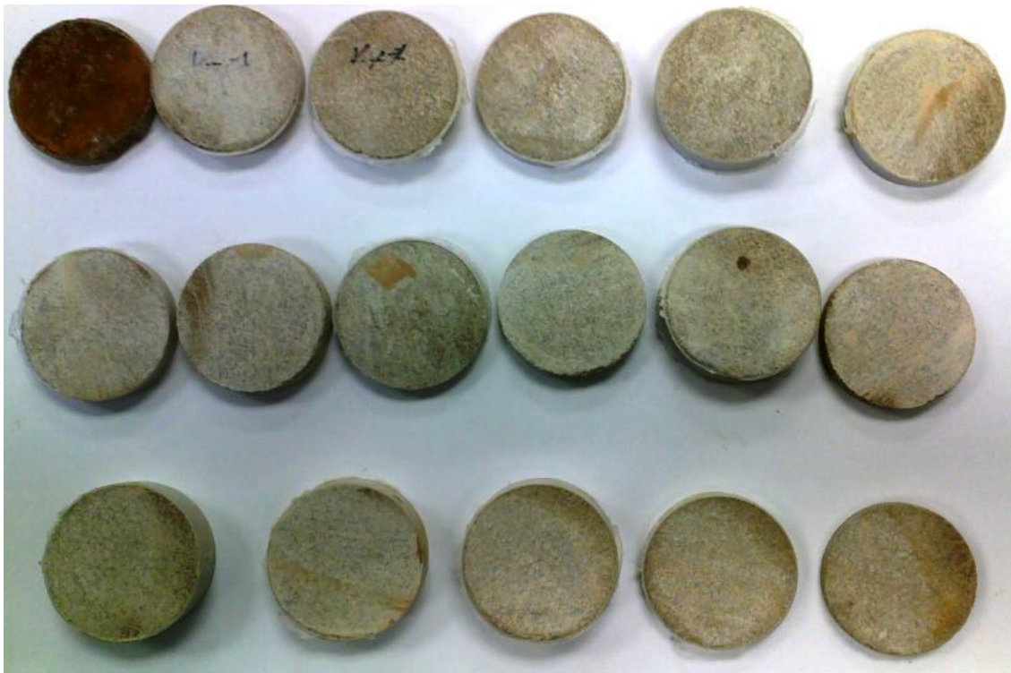
Figure 6.1- Slices of Indiana Limestone core in which no GLDA was flowed. The consecutive inlet faces of the core are shown starting from the top left and continuing on the right
