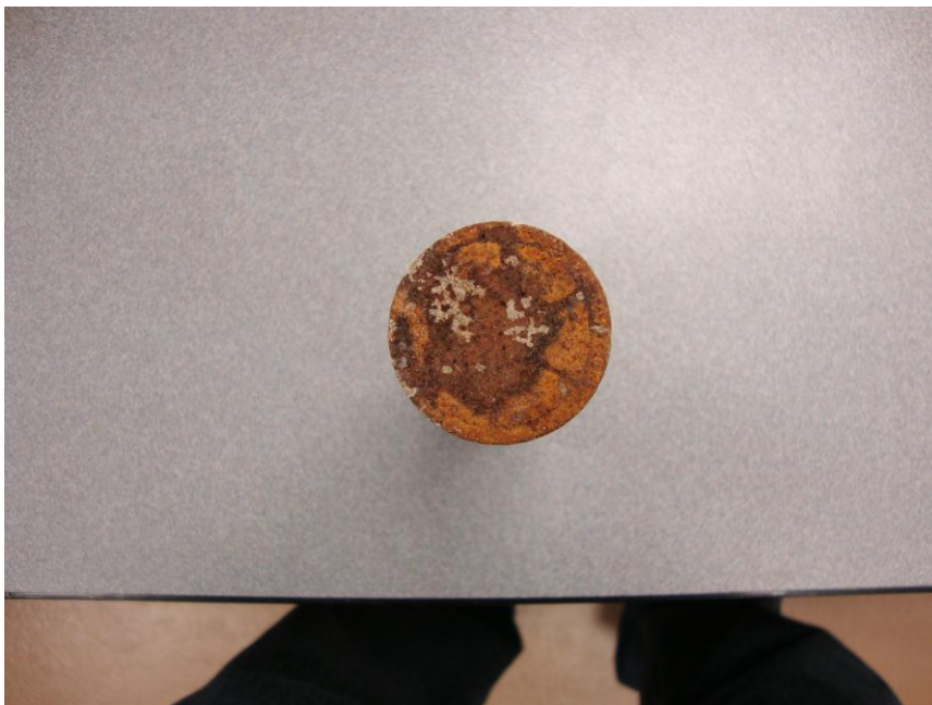
Figure 5.7 – The top view of the core in detail shows formation of small wormhole openings that the CT scan failed to capture
