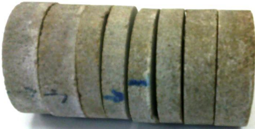
Figure 6.4 – Slices of Indiana Limestone core in which GLDA (2:1 concentration) was flowed stacked together
