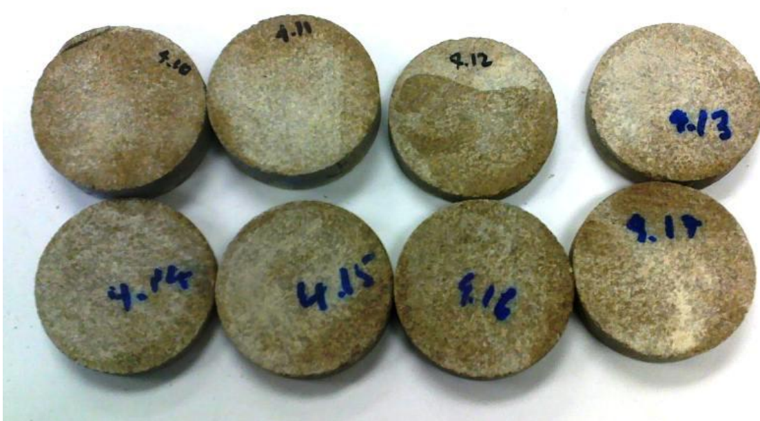
Figure 6.3 – Slices of Indiana Limestone core in which GLDA (2:1 concentration) was flowed with acid at 300°F
