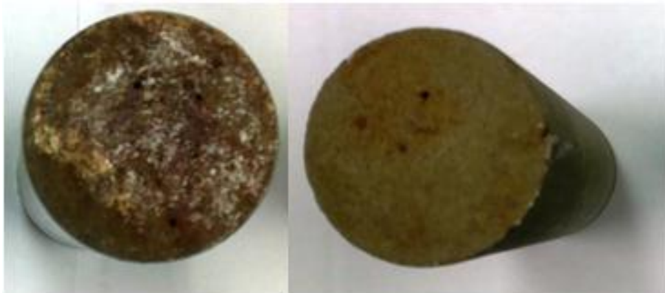
Figure 8.3 – The core on the left had the lower concentration of GLDA (1:1) as compared to the right one (2:1). The core on the right shows a much lower deposit of iron as compared to the left face and thus, a much lower damage
