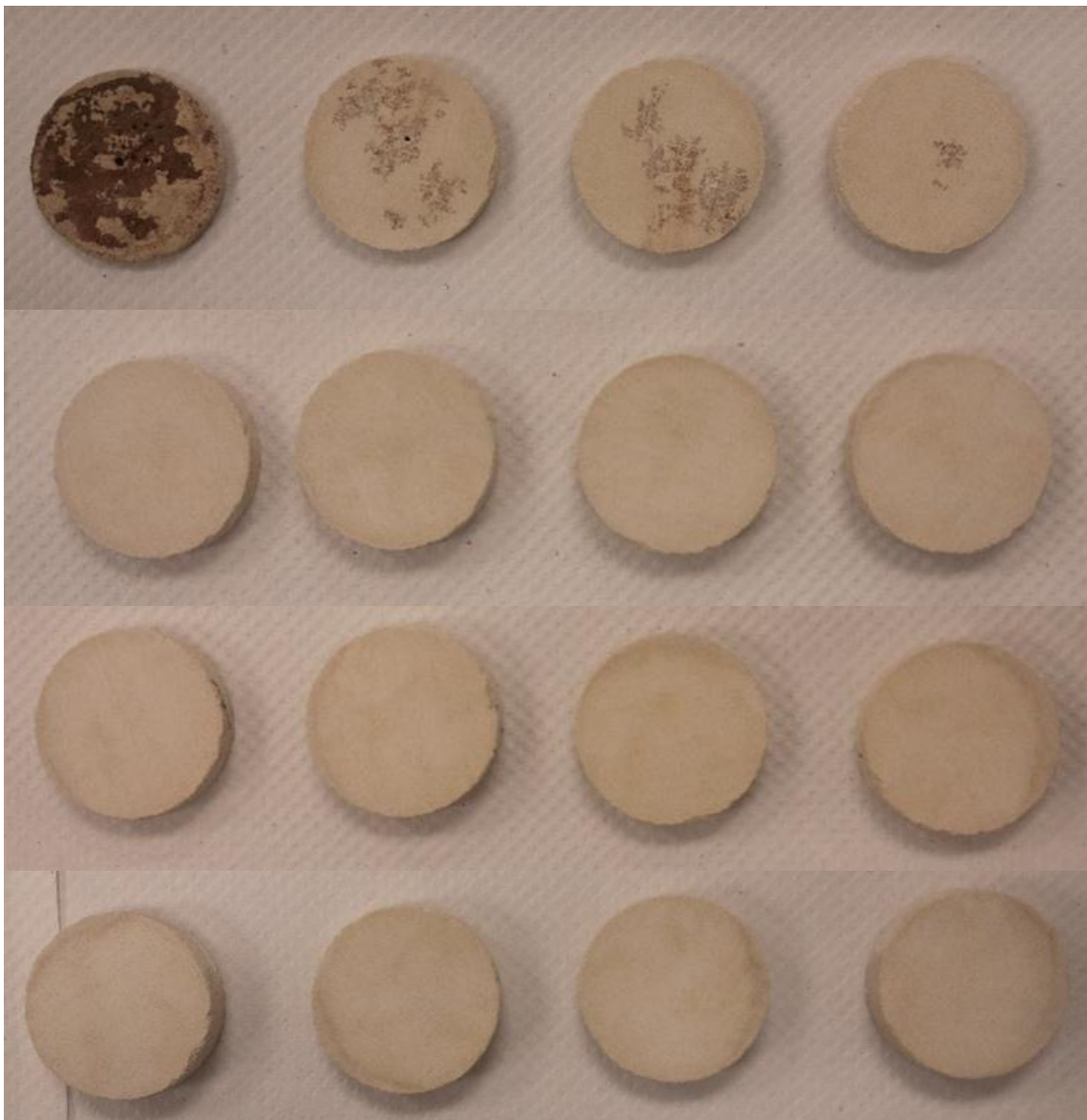
Figure 6.7 – The first 4 core slices show visible marks of iron precipitation in the core in Austin chalk
