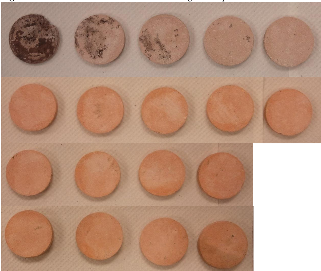
Figure 6.9 – The cut pieces of the Pink Desert core after the treatment
