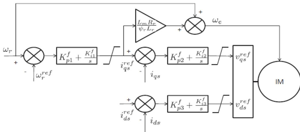
Fig. 3. Flywheel Power Electronics Control
