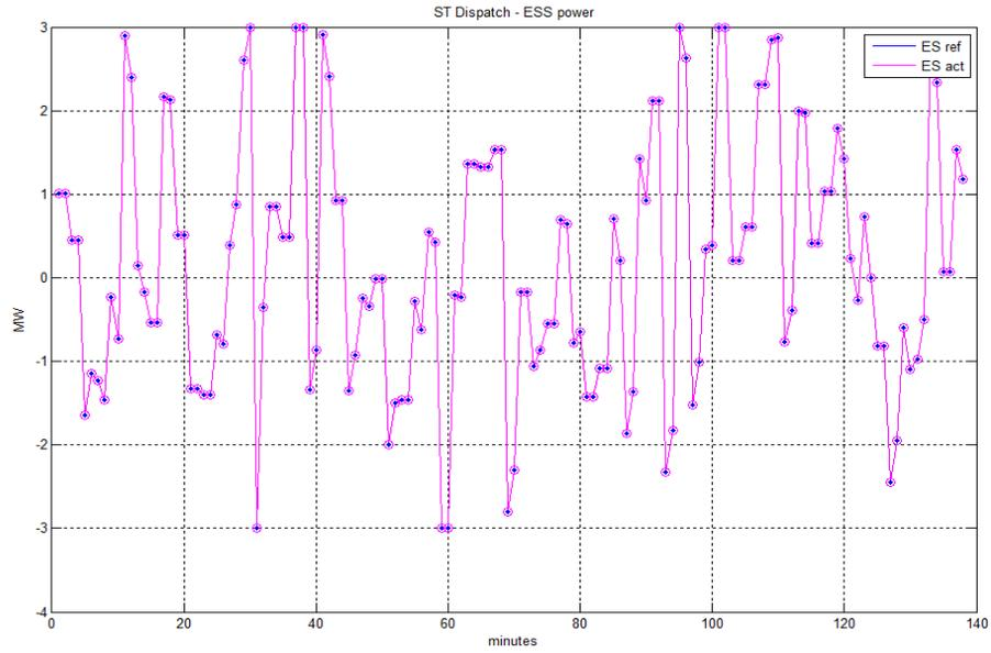
Fig. 6. ESS Power Command and ESS Power Response
