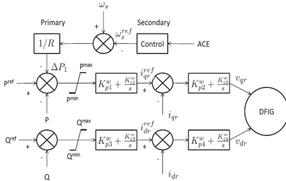
Fig. 2. Wind Generator Power Electronics Control
