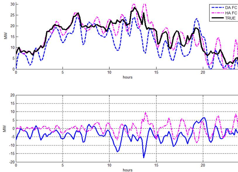
Fig. 10. Power Forecast vs. True Wind Power, Forecast Errors
