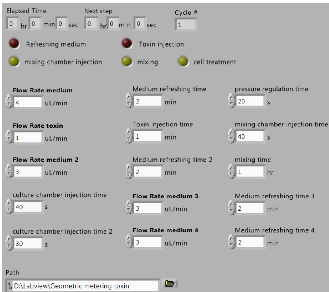
Figure F.3. Front panel of the LabVIEW™ program for microfluidic geometric metering-based live cell toxin screening system (Geometric toxin screening_toxin__20110715.vi).
