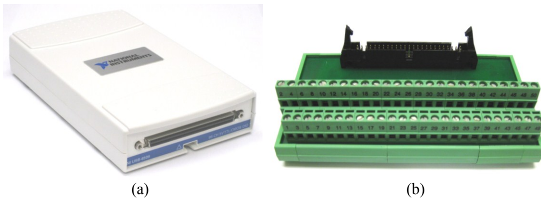
Figure 4.11. Photographs of (a) the NI USB-6509 DAQ and (b) the NI CB-50 connector box.
