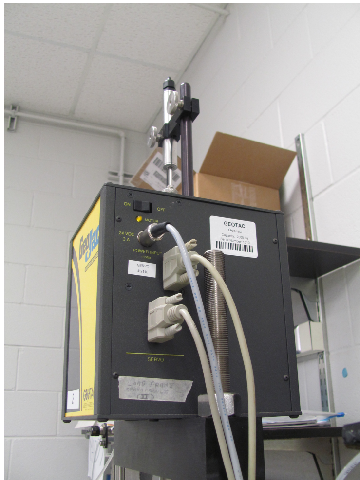
Fig. A.5. Servo module on the side panel of the load frame.
