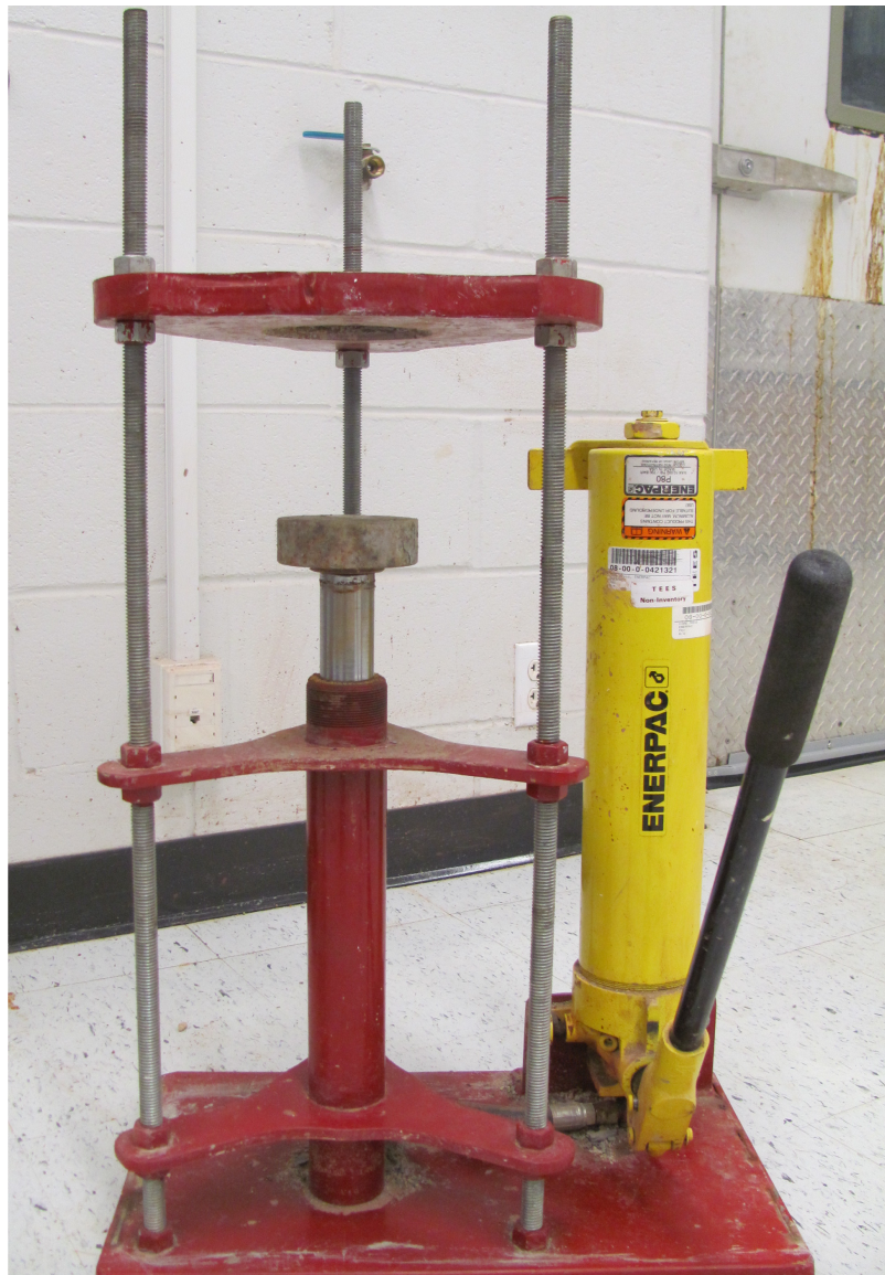
Fig. A.9. Hydraulic hand pump along with the extruder.
