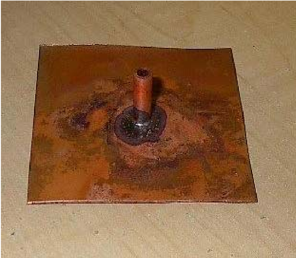
Figure 12. Completed piezometer ring tap
