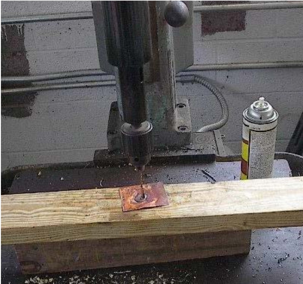
Figure 11. Drilling the 1/8" hole in the copper sheet
