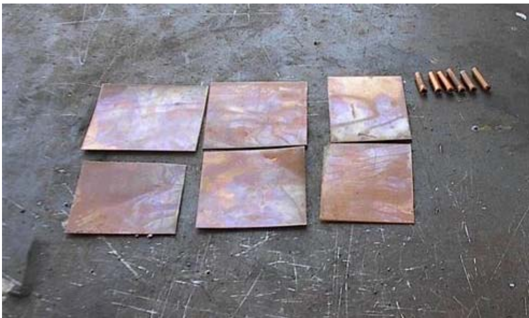
Figure 7. Raw materials for piezometer ring tap
