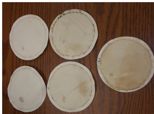
Fig. 37 — Residual \alpha -amylase on filter cake. Enzyme solutions leaving residue on the remaining filter cake after treatment of starch.
