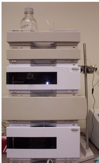
Fig. 6 — HPLC Apparatus. From top to bottom: degasser, quaternary pump, column thermostat, refractive index detector.
