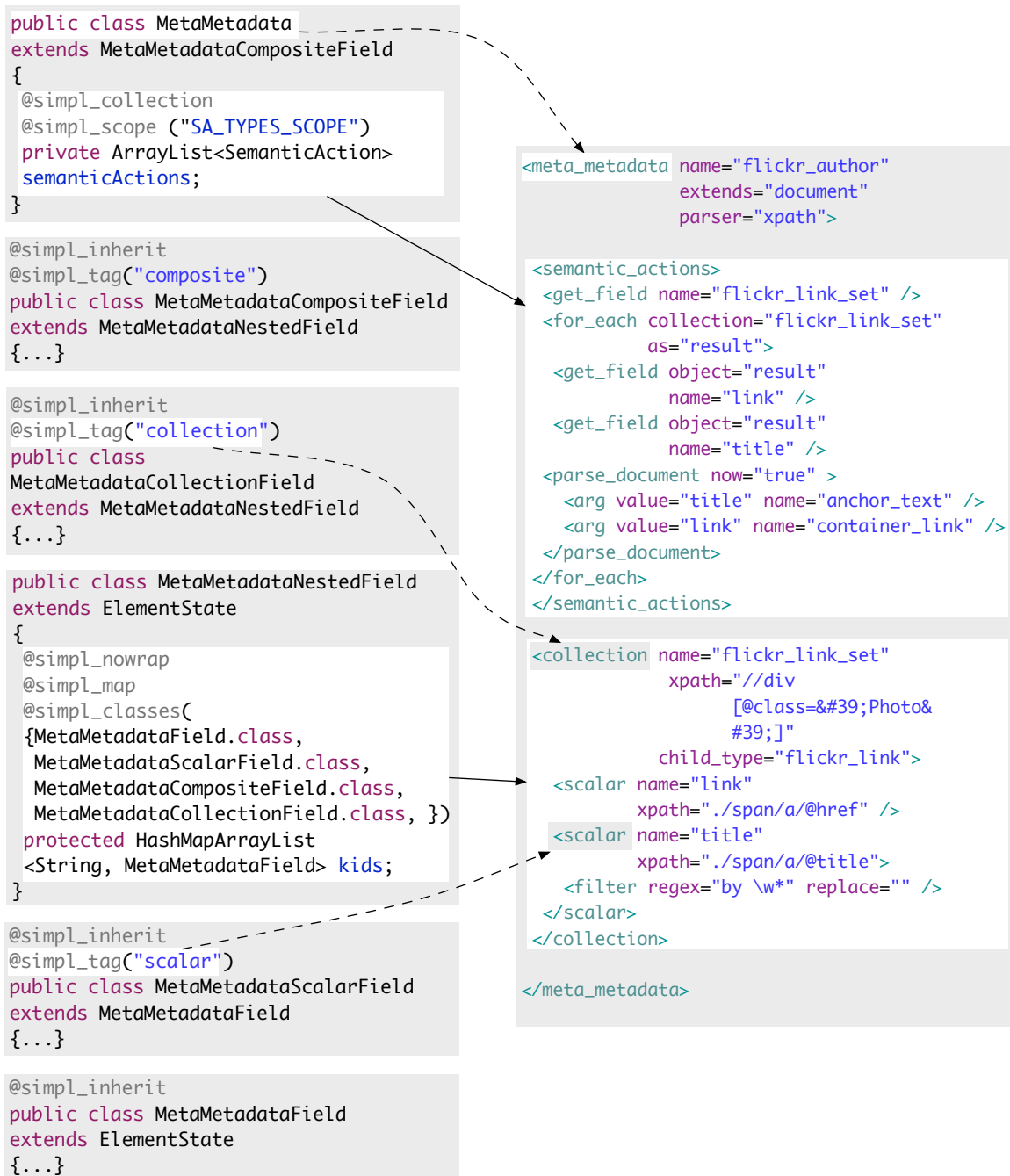
Fig. 29.: The data binding between a meta-metadata wrapper and DBAL-augmented class definitions in Java. S.IM.PL Serialization's support for polymorphic types enables the nested structure of metadata type declarations and semantic actions.
