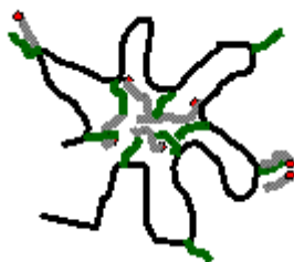
Fig. 22 —Interaction between high surfactant concentrations with multiple hydrophobic modifiers in single polymer molecule.
