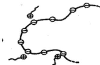
Fig. 18 —Association due to electrostatic attractions between oppositely charged surfactant and polymer molecules.
