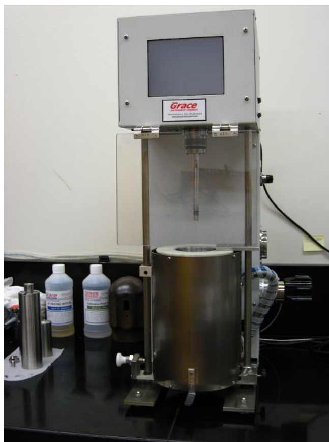
Fig. 59 —High-Pressure / High-Temperature Grace Instrument M5600 Rheometer.
