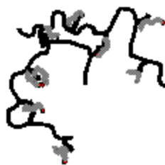
Fig. 21 —Interaction of surfactant with hydrophobically modified polymer.
