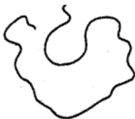
Fig. 17 —Polymer molecule implying no surfactant-polymer interaction.
