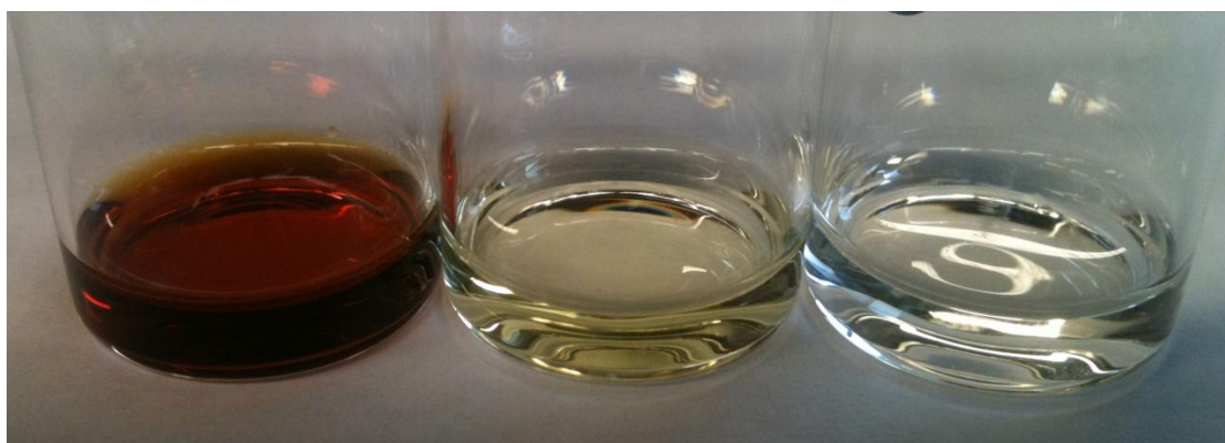
Figure 58. Suspensions of tribosynthesized material from 8,500 cycles on \text{Si}_3\text{N}_4 (left), 8,500 cycles on Si (center) and 5,000 intermittent cycles on Si (right).
