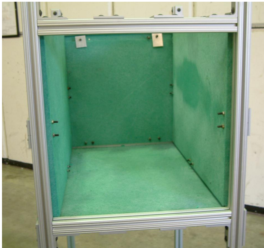
Figure 22. Borated-polyethylene shielding cart designed to reduce neutron transmission during the irradiation of bismuth-209 with alpha-particles.
