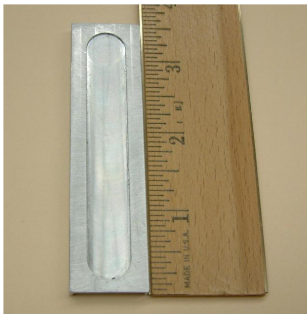
Figure 23. Aluminum target with groove designed to dissipate heat produced during the bombardment of melted bismuth.
