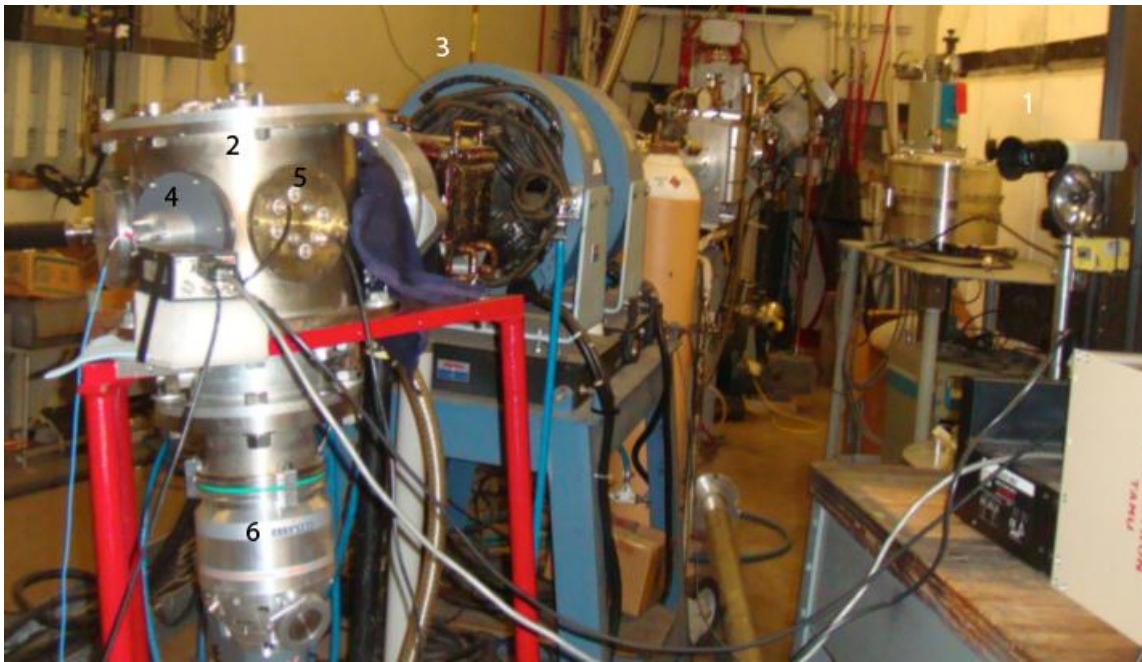
Figure 9. External target system utilized for the production of At-211. 1) Camera system. 2) Housing of target system. 3) Focusing magnet. 4) Target holder. 5) Faraday cup connections. 6) Vacuum system.
