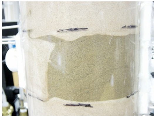
Figure 4.3 - Time series photographs of the upper lenses in the lens column (top) and the killed-controlled column (bottom). The progressive development of a sharp redox interface in the lens column is marked by reddish iron oxide bands.
