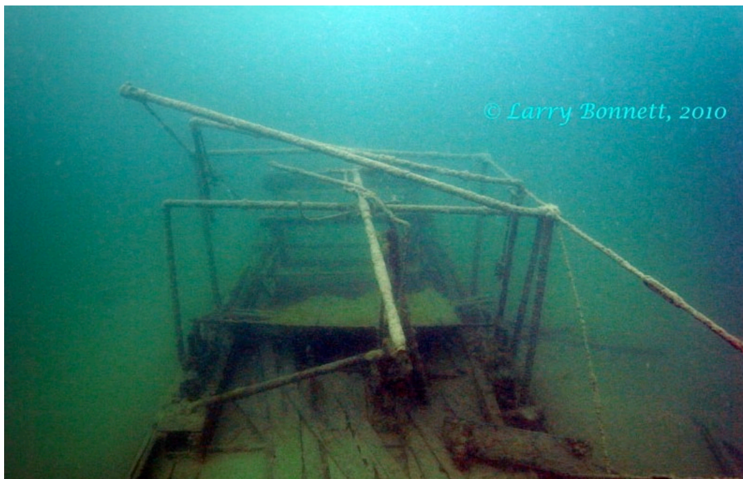
FIGURE 3.6. Damage to the hogging system in the stern (Photo by Larry Bonnett).
