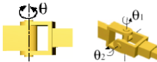
Figure 10. The ‘R’ revolute joint and the ‘T’ joint or the universal joint
