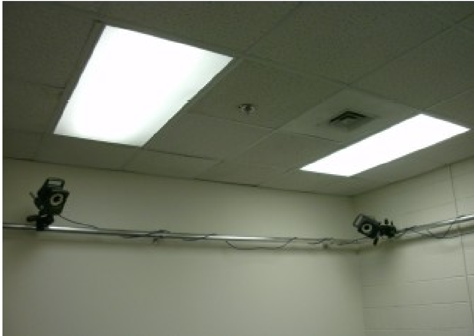
Figure 21. Set up of infrared detection cameras in VICON motion capture system
