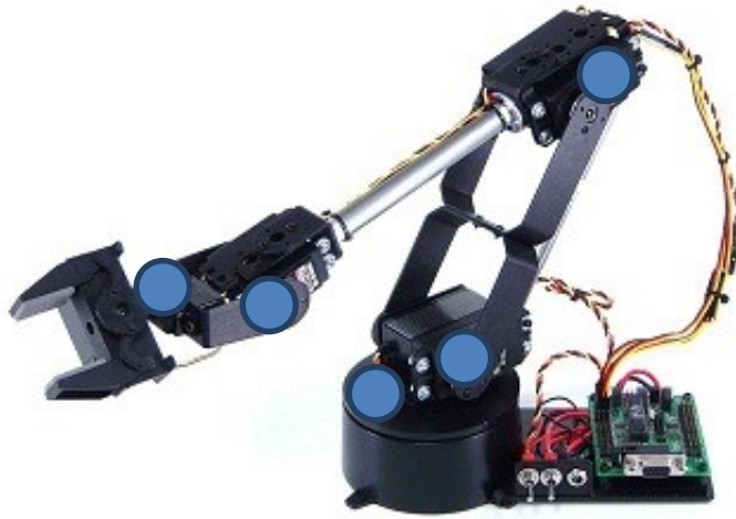
Figure 20. Robot arm with infrared markers fixed at different joints
