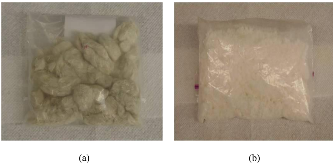
Figure 11. Alumina fibers (a) Nextel™ 720 (b) ALBF1.
