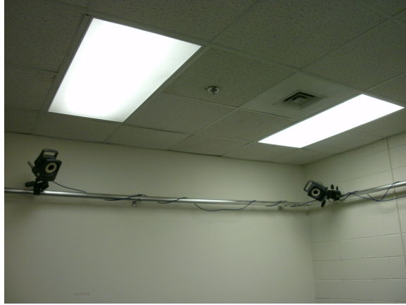
Fig. 12. VICON motion capture system consisting of infrared cameras.
