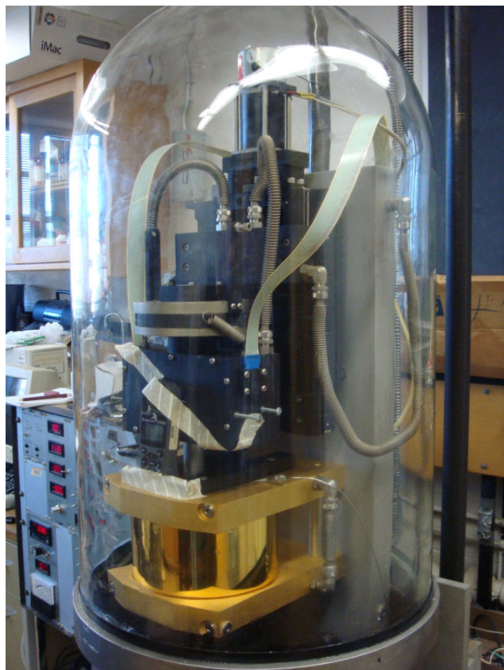
Figure 8. Image of the HTT used in these experiments, depicting the heating element and glass bell jar.
