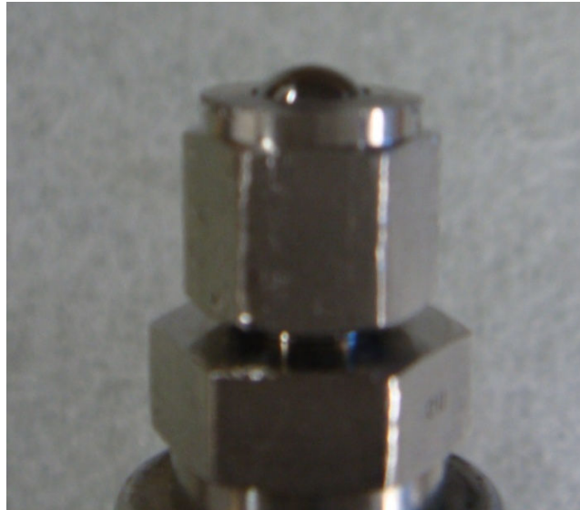
Figure 11. Ball bearing shown bolted in place on the load shaft.
