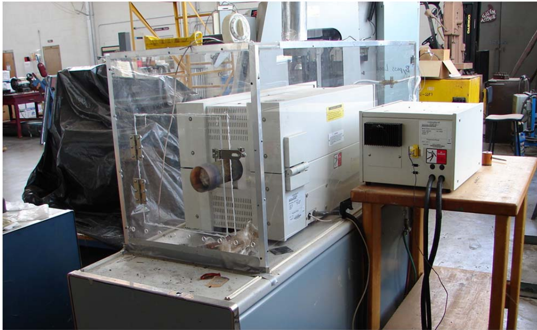
Figure 2. 2 Blue-M CVD furnace used for MWCNT coating of various substrates.
