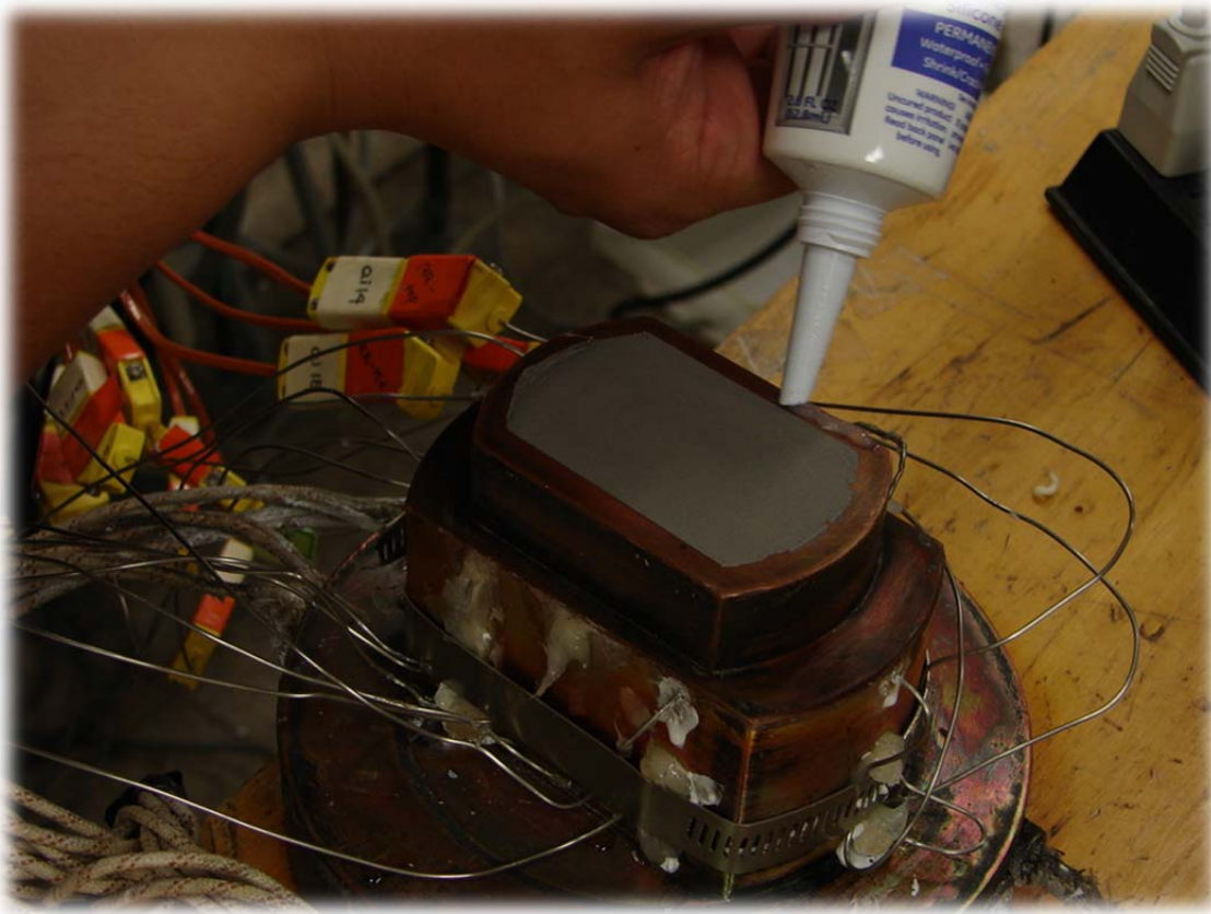
Figure A.14 Applying silicon at the edge of the thermal paste coated copper block.
