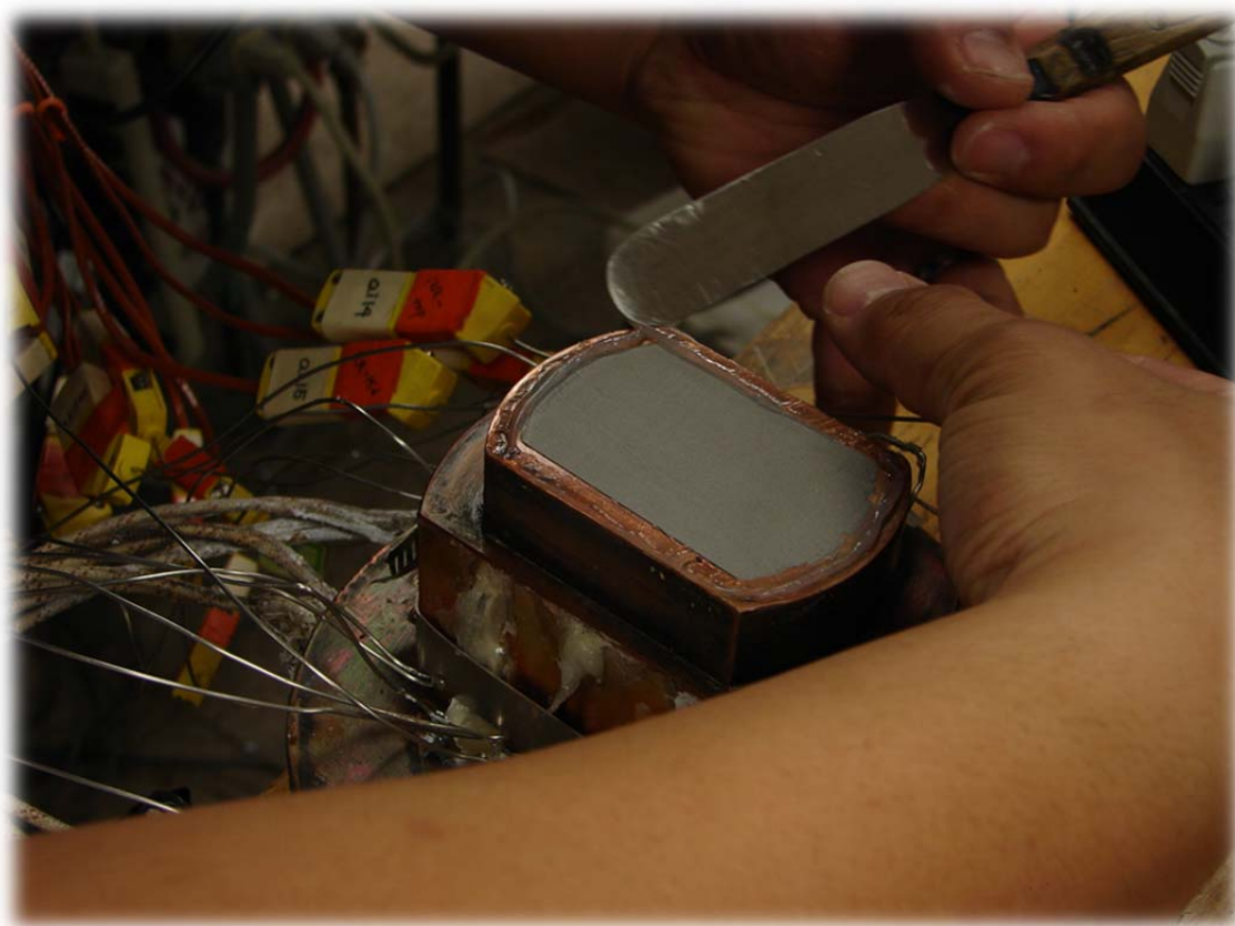
Figure A.16 Spreading the silicon around the perimeter.
