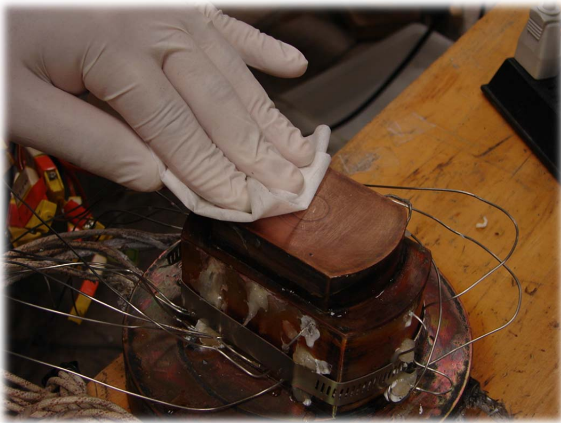
Figure A.2 Surface cleaning.
