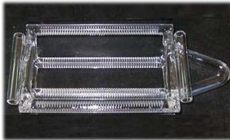
Figure 2. 19 Quartz boat to load 3” wafers.
