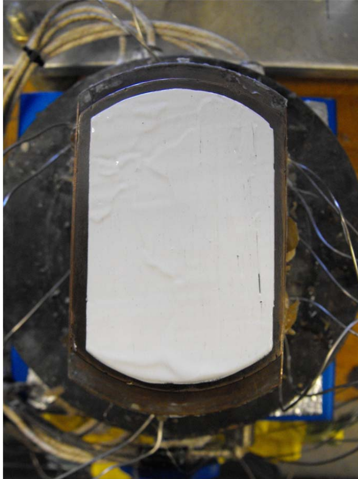
Figure 2. 5 Thermal paste on the copper block.
