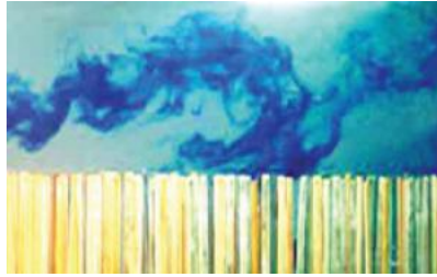
Fig. 21. Dye visualization of vortex above rigid canopy (from Ghisalberti et al. 2009).
