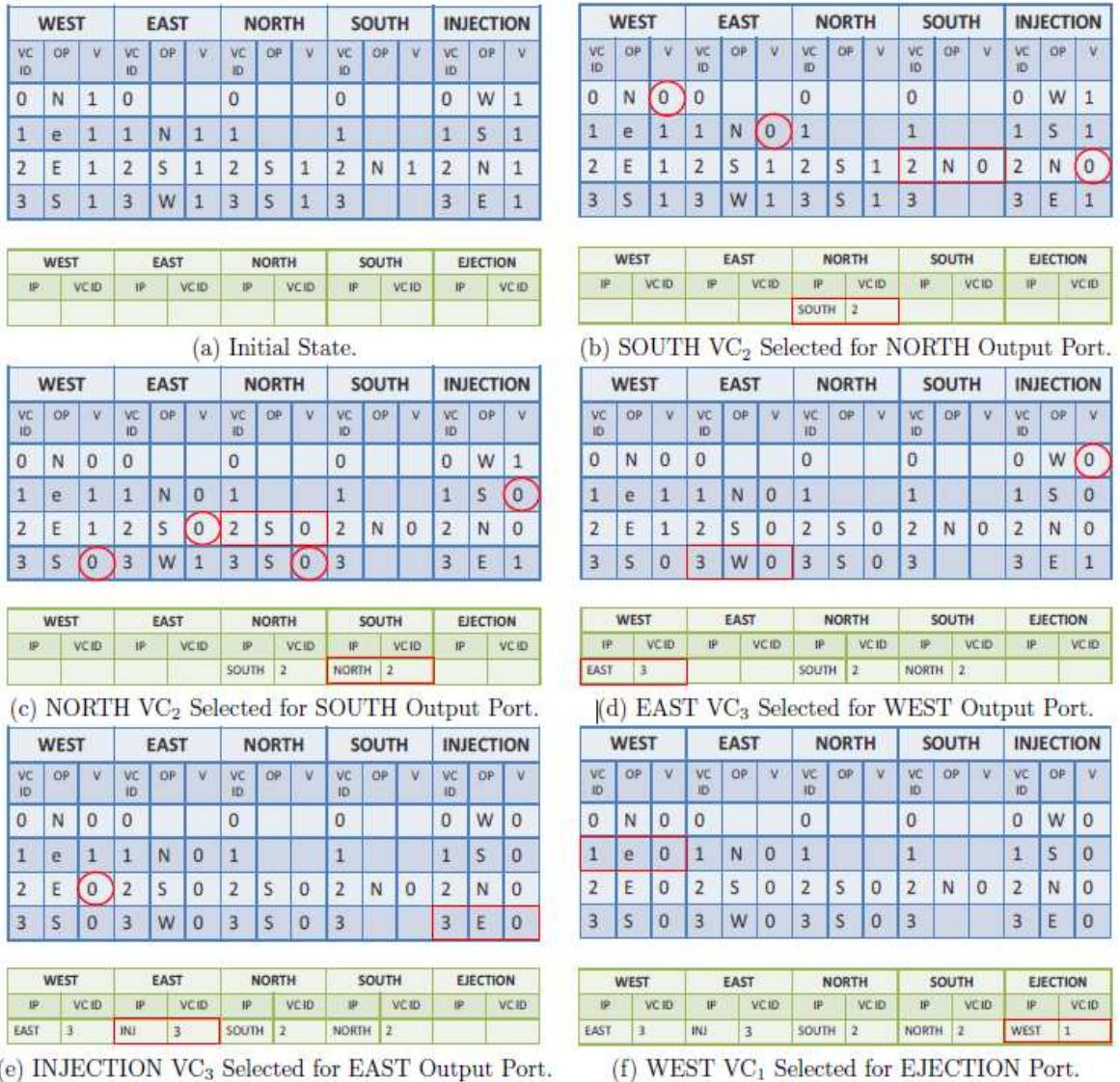
Figure 14. Walkthrough Example. (a) VCCT and DGT record the states of all requests, where all fields of DGT are empty. (b) SOUTH VC 2 is granted to DGT. In the mean time, we invalidate VC 0 of WEST input port, VC 1 of EAST input port and VC 2 of INJECTION port. (c) NORTH and EAST have the same amount of valid requests. Here we assume NORTH input port is the diversity port. VC 2 is selected and SOUTH field of DGT is filled. We invalidate other requests which destined to the same direction. (d), (e) and (f) follow the same rules.
