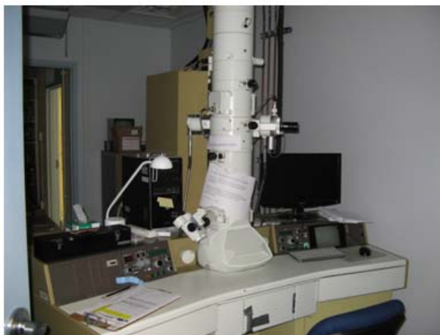
Figure 37 JEOL 1200EX TEM used for NP/amino acid morphology characterization
