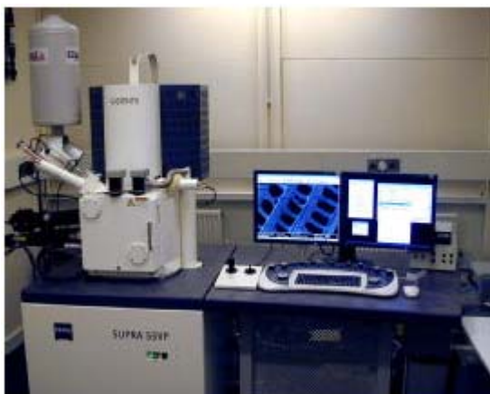
Figure 32 Supra 55 scanning electron microscope (SEM) equipped with energy dispersive X-ray spectroscopy (EDS) (128)
