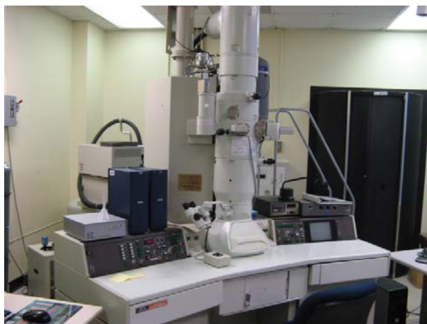
Figure 36 JEOL-JEM 2010 TEM used to characterize the morphology of the NP/ CNS of the cockroach
