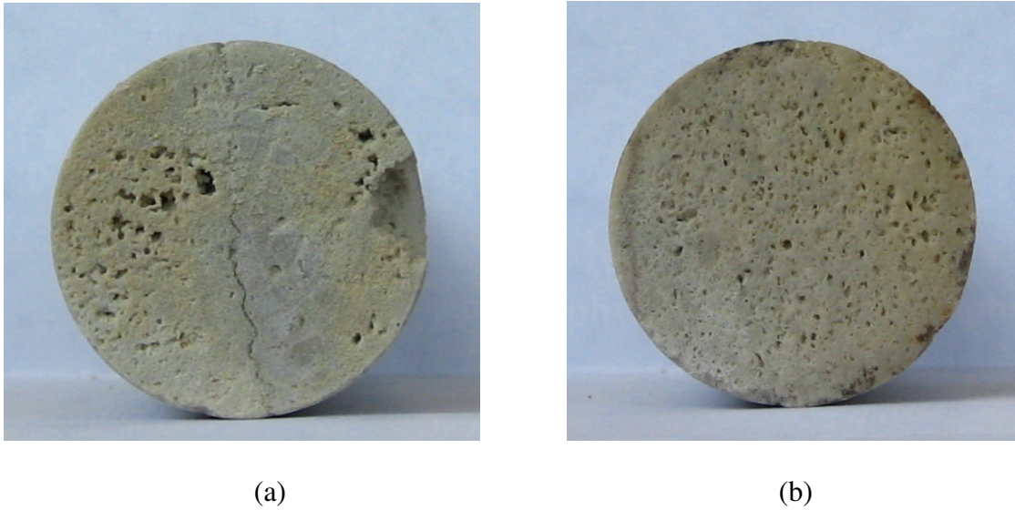
Fig. 5.12: Dolomite core inlet (a) and outlet (b) after acid injection. Test was conducted at 1 \text{ cm}^3/\text{min} and 200^\circ\text{F} .
