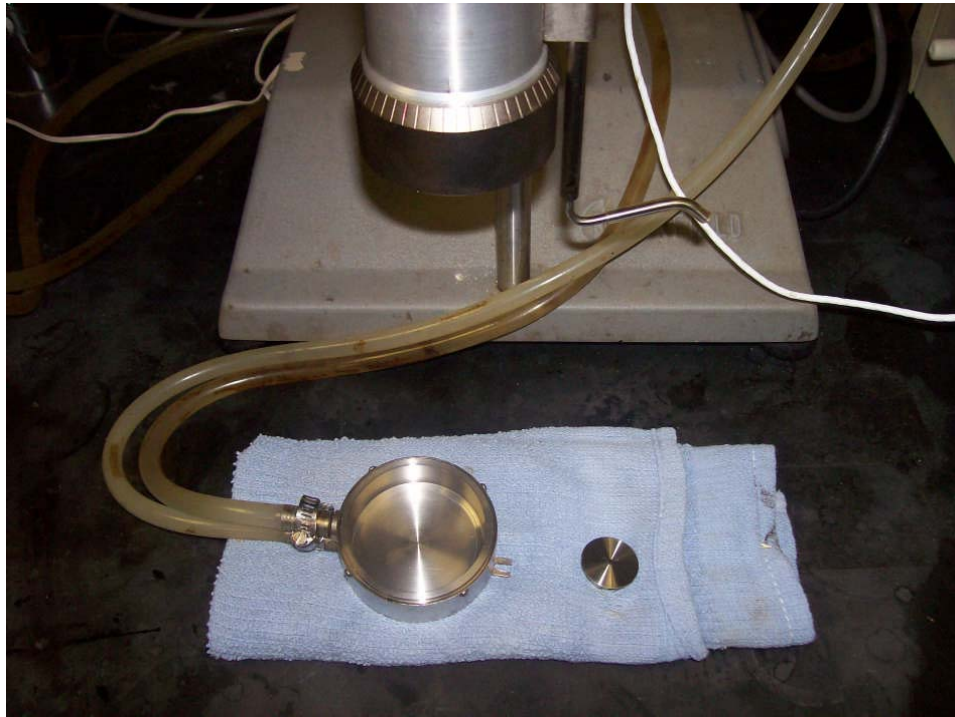
Fig. 3.9 Photograph of the spindle (to the right) and container (to the left) where it rotates.
