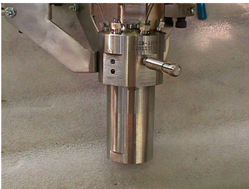
Fig. 3.3 Reaction vessel is assembled to the cover fixed in the supporting shelf.
