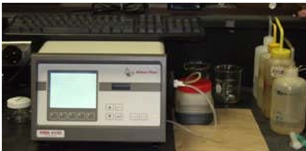
Fig. 3.11 Photograph of the density meter.
