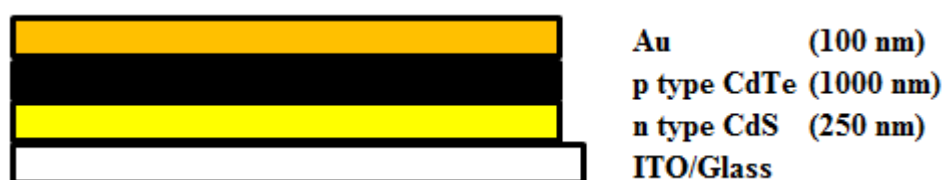
Fig. 26. The superstrate configuration of a thin film CdTe solar cell.
