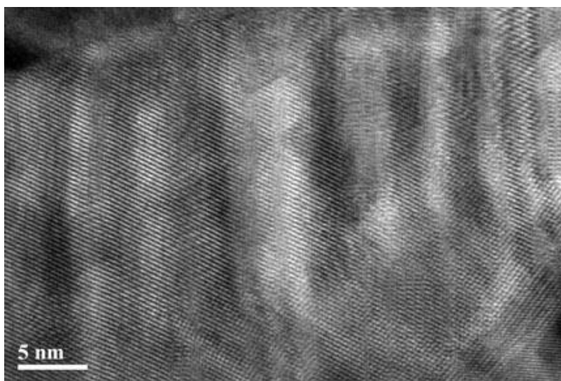
Fig. 62. Cross-sectional TEM image of defects in CdS.
