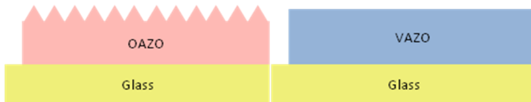
Fig. 14. Structure of the OAZO single layer (left) and the VAZO single layer (right).
