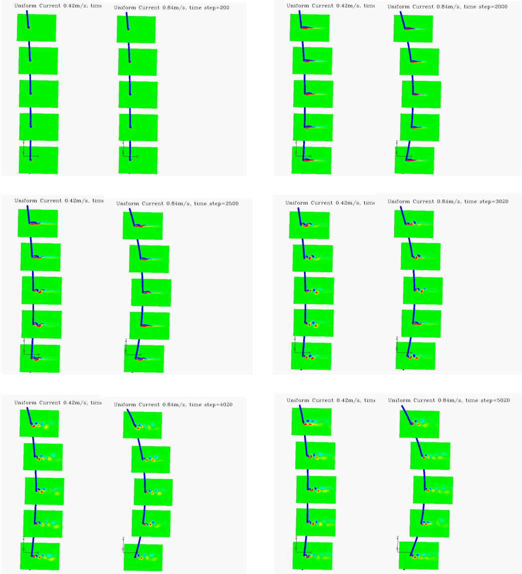
Fig. 33 Vortex Shedding Evolution, Left: U=0.42 m/s, Right: U=0.84 m/s
