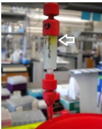
Figure 2-4. CysM Ni-IMAC column during CysM purification. This image shows the yellow band (indicated with a white arrow) at the top of the nickel column which indicated that the CysM protein was bound.
