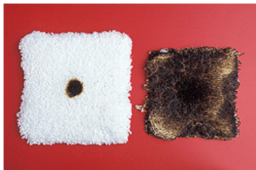
Figure 2.13. Images of 50/50 cotton polyester blend carpet with (left) and without (right) FR treatment after pill test. 187
