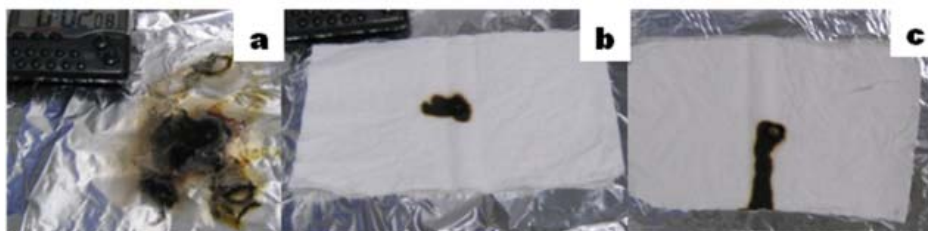
Figure 4.8. Pill test images of post-burn control fabric (a), 10 BL AP/(-) POSS coated fabric (b), and 10 BL of (+)POSS/(-)POSS coated fabric (c). 232
