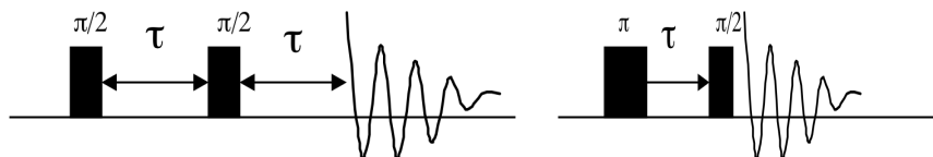
Figure 2.2. Solid echo pulse sequence (left) [ 90_y^\circ\text{-}\tau\text{-}90_x^\circ\text{-}\tau\text{-acquire} ] (left); inversion recovery pulse sequence (right) [ 180^\circ\text{-}\tau\text{-}90^\circ\text{-acquire} ] (right).
