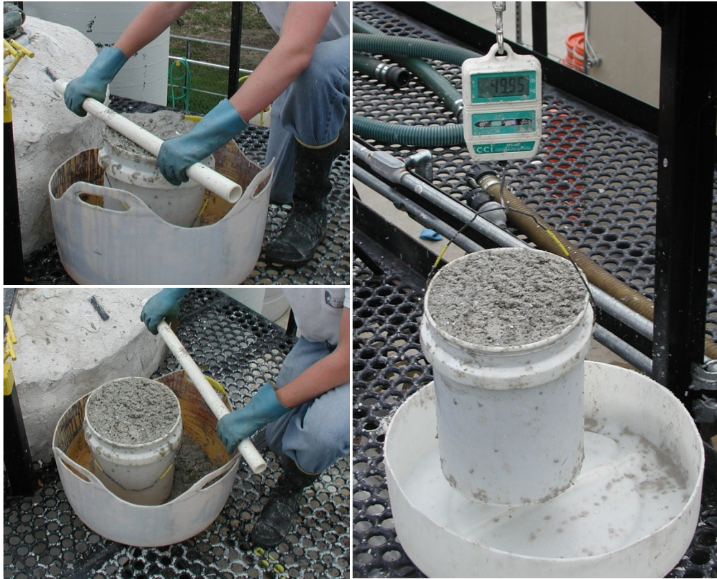
Figure 3-1. Five-gallon bucket being used to measure the density of fermentation slurry at pilot plant.
