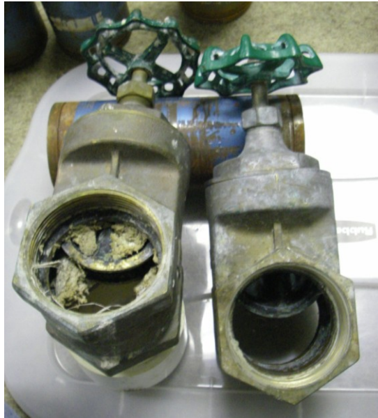
Figure 2-22. Two 3-inch gate valves that were removed from fermentor recycle loops because biomass jammed valve in position shown.
