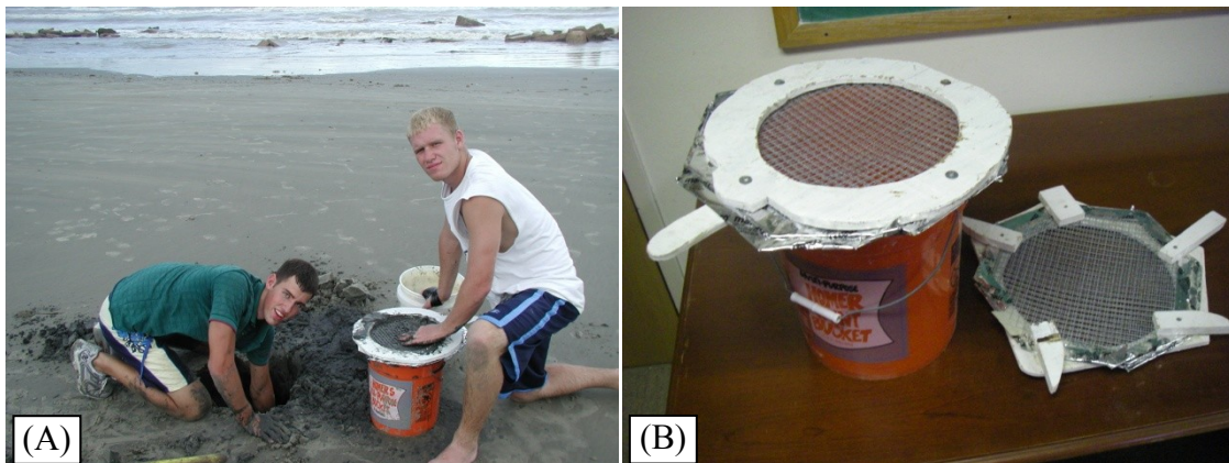
Figure 2-11. (A) Picture of student workers collecting and screening sand from Galveston, TX beach. (B) Bucket-top screens used to eliminate large particles (e.g., shells, debris) that could damage pumps.
