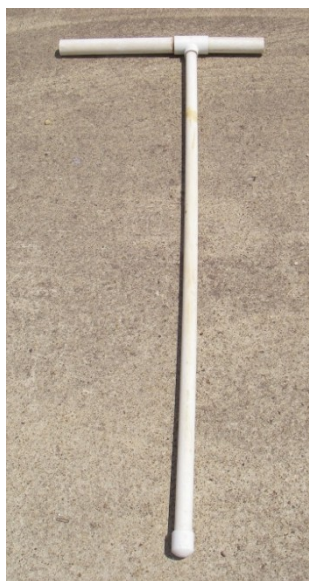
Figure 2-28. Picture of T-shaped leveling tool made from PVC piping.
