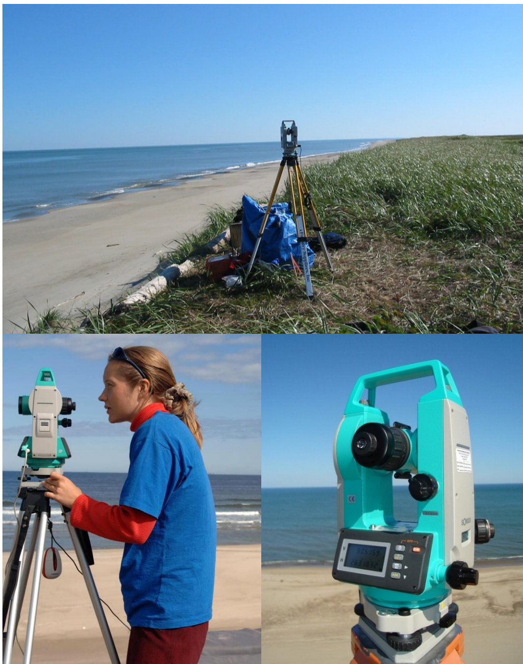
Figure 3. Lietz/Sokkisha Model DT5A and DT5 theodolites were used to monitor the movement patterns of gray whales.
