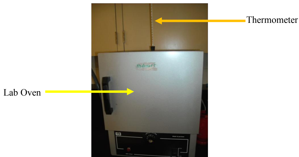
Figure 15: Oven used for drying carbon nanotubes
