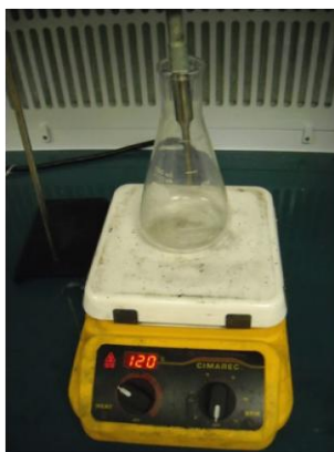
Figure 12: Sonicator probe inserted inside glass beaker, placed on hot plate
