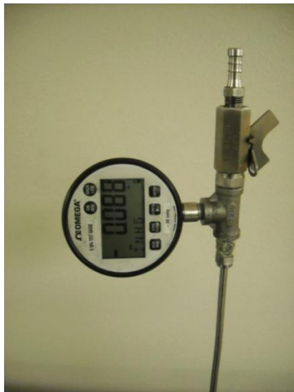
Figure 9: Pressure gauge connected to vacuum pump
