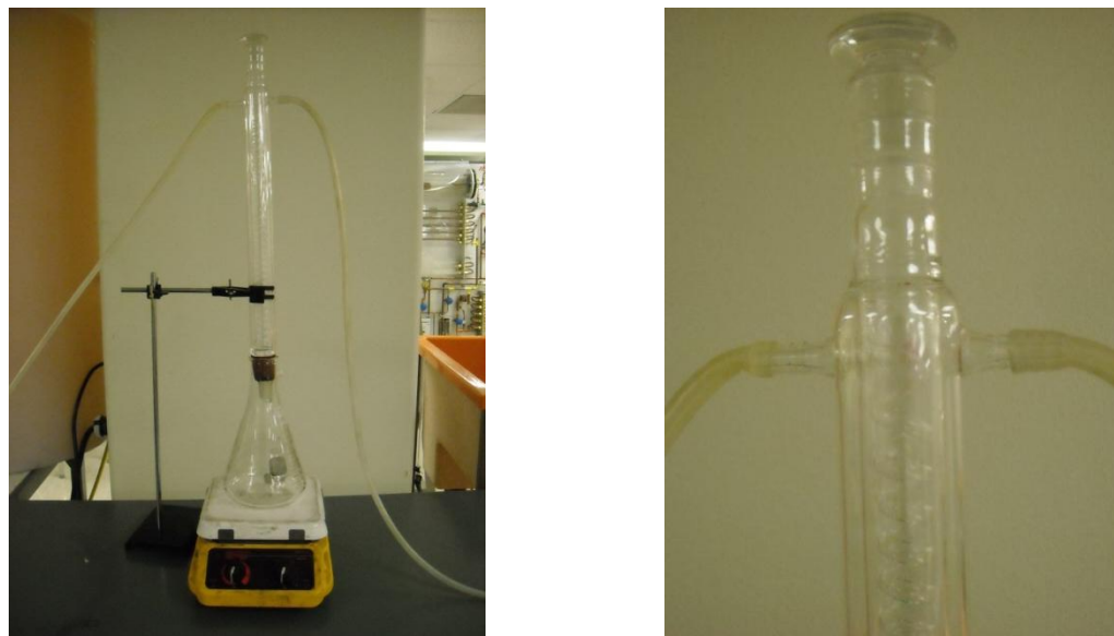
Figure 13: a) Acid treatment process b) Reflux condenser with tubing
