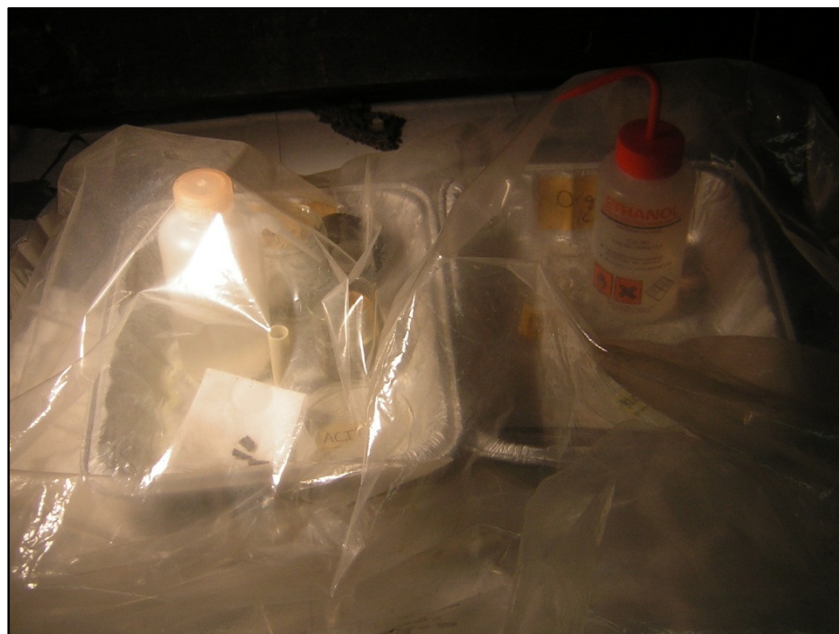
Figure 3-2: Glovebag acid wash station.
