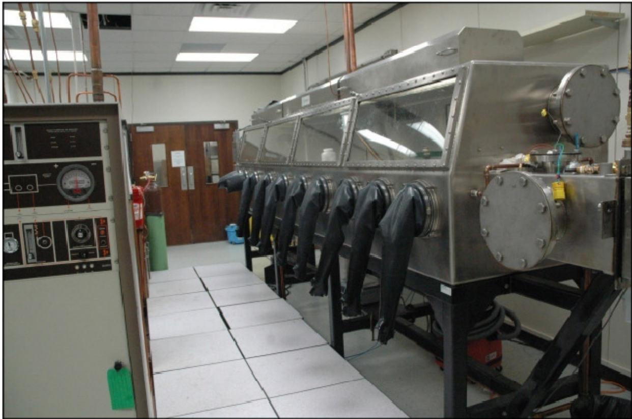
Figure 3-1: Large inert atmosphere glovebox used for handling of pyrophoric uranium powder.
