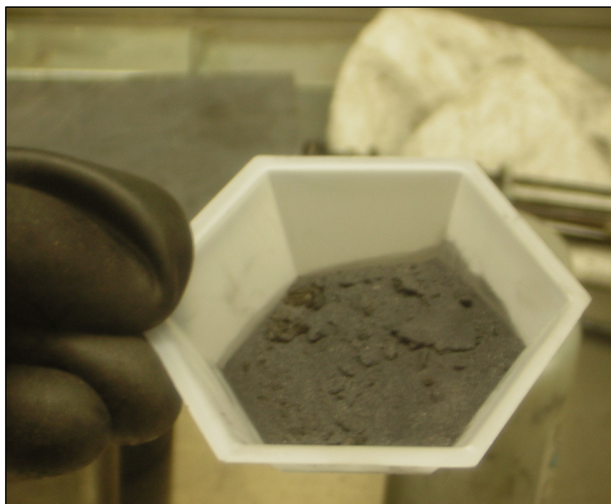
Figure 3-8: DU powder produced by the hydride/dehydride process.
