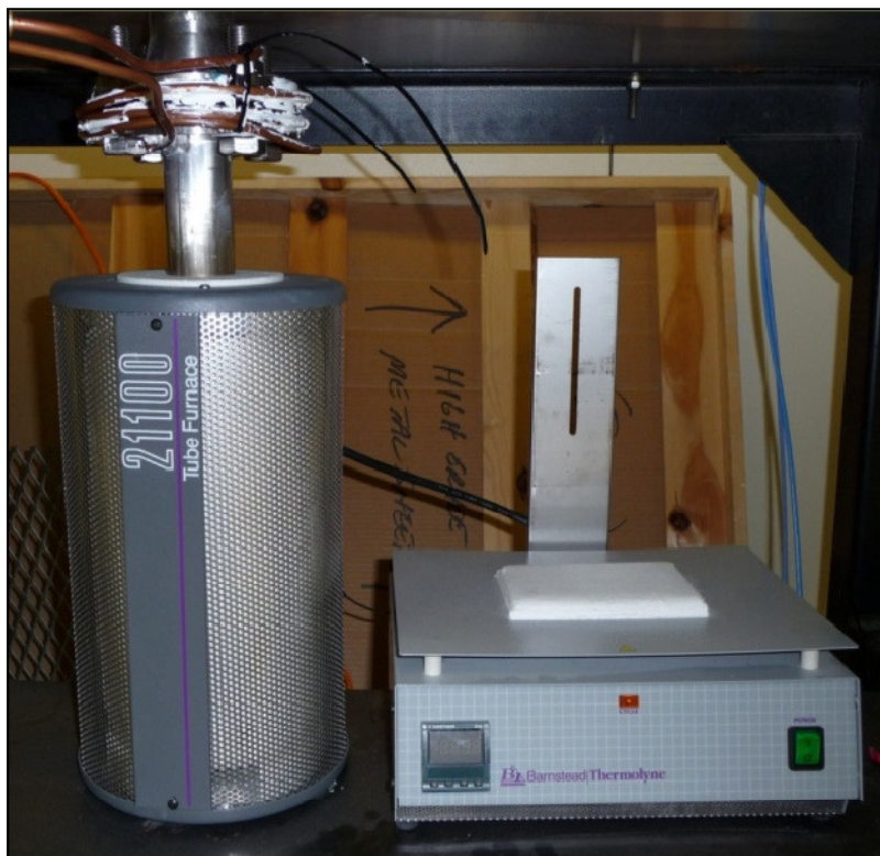
Figure 3-6: Furnace used for hydride/dehydride process.
