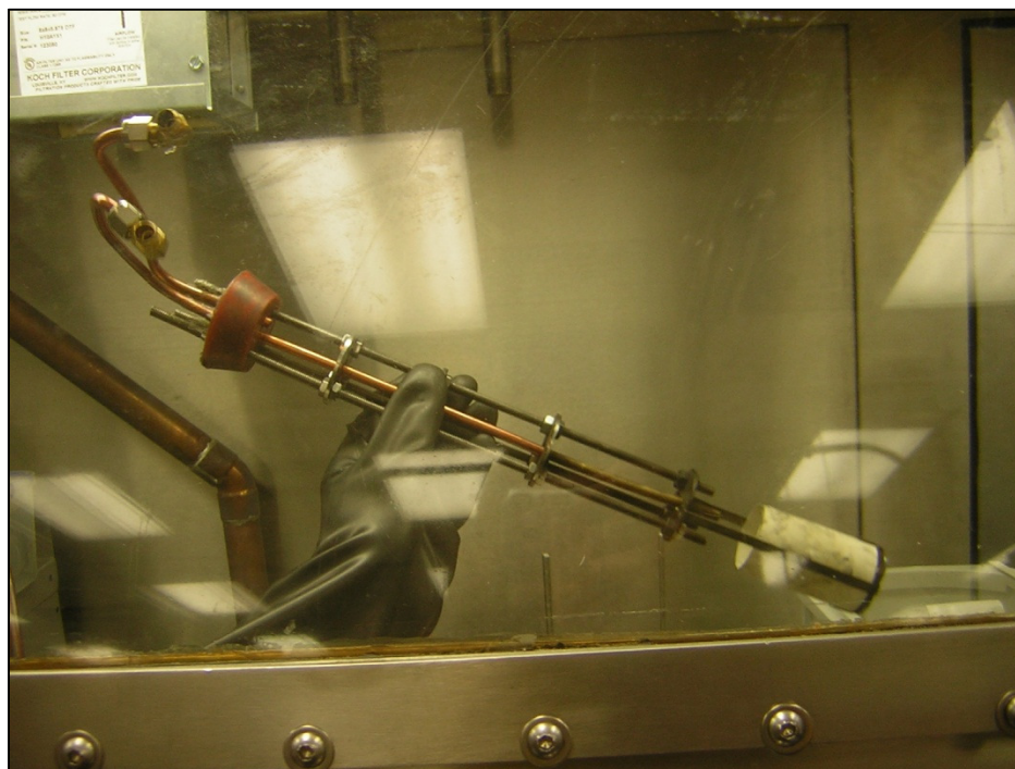
Figure 3-4: Hydride/dehydride well insert used for uranium powder production.
