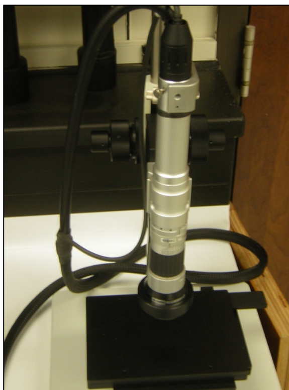
Figure 3-10: Hirox KH-1300 Digital Microscope used for powder imaging.
