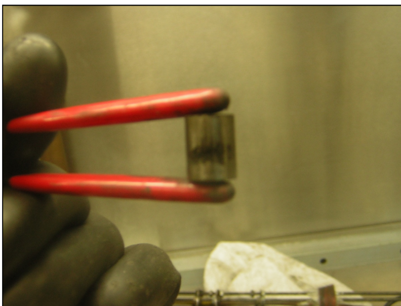
Figure 4-3: Pellet 3 as pressed, before sintering.
