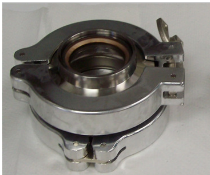
Figure 3-9: Atmospheric Containment Vessel (ACV) used for powder transfer.
