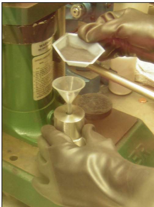
Figure 3-11: Loading powder into dual-action punch and die for compaction.
