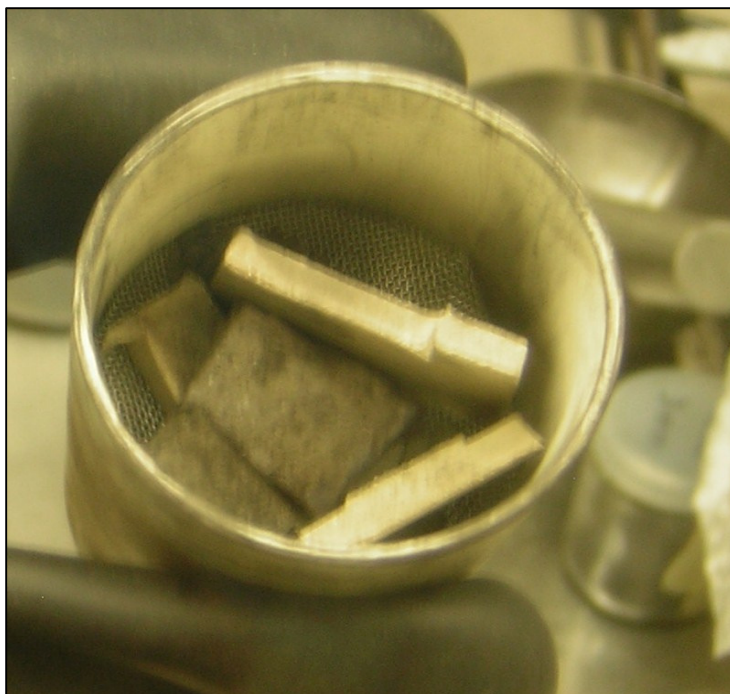
Figure 3-5: DU coupons loaded into yttria crucible for hydriding.
