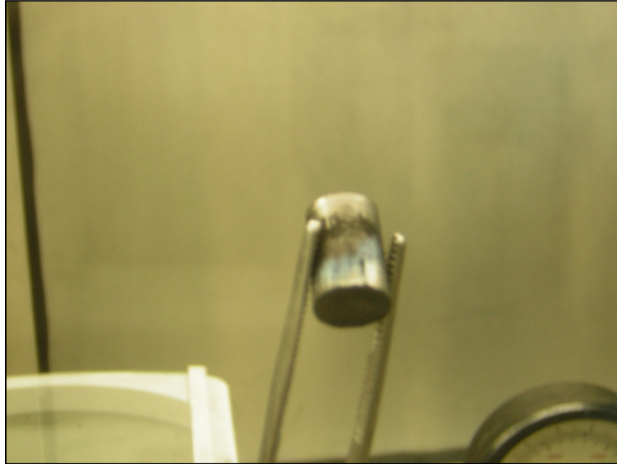
Figure 4-5: Pellet 4 after sintering.
