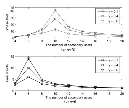
Fig. 7. The time spent to attain the desired state by the negotiation-based sensing policy against the number of SUs with different γ's. (a) The case with n = 10.
