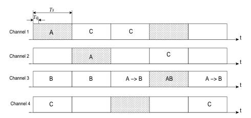
Fig. 14. Illustrations of our proposed opportunistic MAC protocol. The shadowed rectangles represent the time slots during which the PUs are active. The empty rectangles represent the unused time slots. Let A, B, and C be three SUs. If A wants to send packets to B, A follows the B's hopping sequence to meet with it and exchange the negotiation packets if the channel is unused by the PUs.
