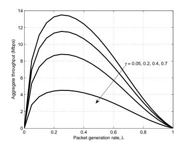
Fig. 17. The aggregate throughput of SUs against the packet generation rate. The average packet size is set to 170 bytes. The number of SUs N = 20. gamma is set to 0.05, 0.2, 0.4 and 0.7, respectively.
