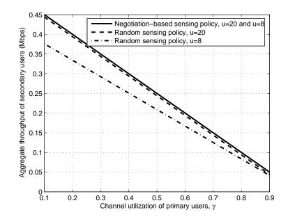
Fig. 12. The aggregate throughput  $(\eta)$  of SUs varies with different channel utilization  $(\gamma)$  of PUs when the number (u) of SUs is equal to 20 and 8. The system utilization  $(\rho)$  of SUs is 0.1 and the number (n) of licensed channels is 5. The solid line represents the negotiation-based sensing policy for both u = 8 and u = 20, the dashed line represents the random sensing policy with u = 20, the dashed line represents the random sensing policy with u = 8.
