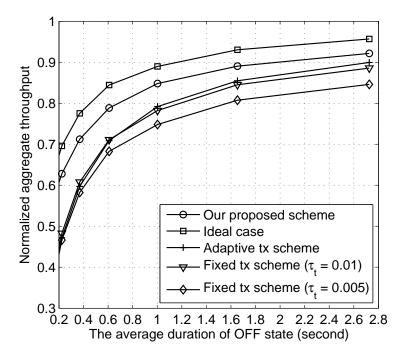
Fig. 36. The normalized aggregate throughput vs. the average duration of OFF state when the PUs' activity follows the lognormal distribution.
