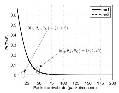
Fig. 49. The probability that the HOL delay is larger than 6 frame periods when the packet arrival rate varies and the average SNR ( $\overline{\gamma}$ ) is 10 dB.
