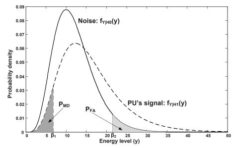
Fig. 24. The illustration of the relationship between the  $P_{FA}$  and  $P_{MD}$  in the two-threshold sequential sensing. The two thresholds  $\beta_1$  and  $\beta_2$  control  $P_{MD}$  and  $P_{FA}$ , respectively.
