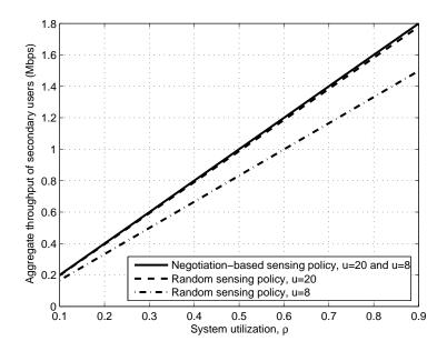
Fig. 10. The aggregate throughput  $(\eta)$  of SUs against different system utilization  $(\rho)$  of SUs when the number (u) of SUs is equal to 20 and 8. The channel utilization  $(\gamma)$  of PUs is 0.6, and the number (n) of licensed channels is 5. The solid line represents the negotiation-based sensing policy for both u = 8 and u = 20, the dashed line represents the random sensing policy with u = 20, the dashed line represents the random sensing policy with u = 8.
