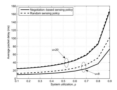
Fig. 9. The average packet transmission delay  $(W_s)$  against the system utilization  $(\rho)$  of SUs with different number of SUs (u) when the channel utilization  $(\gamma)$  of PUs is 0.6. The number (n) of licensed channels is 5. The solid lines represent the average packet transmission delay under negotiation-based sensing policy, and the dashed lines represent the average packet transmission delay under the random sensing policy.
