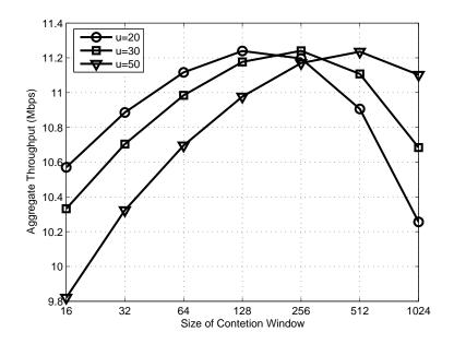
Fig. 26. The aggregate throughput against the size of contention window  $(CW_{min})$ . The number (n) of sensors is set to be 4. The channel utilization  $(\gamma)$  of PUs is set to be 0.5.  $R_c$  and  $R_d$  are set to be 1 Mbps.
