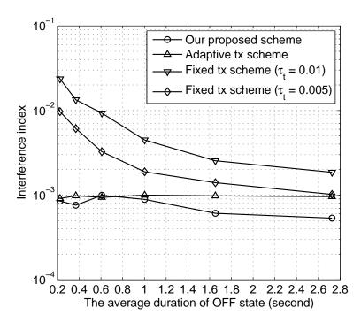
Fig. 37. The interference index vs. average duration of OFF state when the PUs' activity follows the lognormal distribution.
