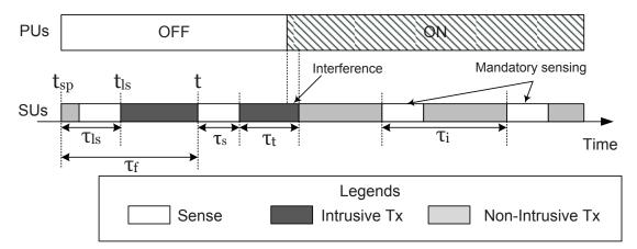
Fig. 32. Illustration of our proposed spectrum access schemes. The transmission duration  $\tau_t$  depends on  $\tau_f$  and the interference constraints. The SUs may interfere with the PUs when both the SUs and PUs access the spectrum.
