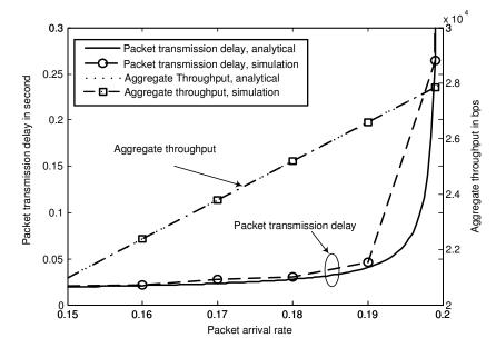
Fig. 30. Analytical and simulation results for the non-saturation network case when the packet arrival rate varies. The number (u) of contending SUs is set to be 10, the number (n) of licensed channels is set to be 4, the channel utilization  $(\gamma)$  of PUs is set to be 0.5.
