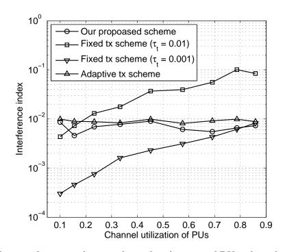
Fig. 41. The interference index vs. channel utilization of PUs when the PUs' activity follows the gamma distribution.
