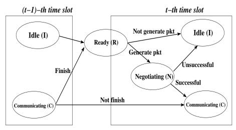
Fig. 15. The diagram of node states transition from (t-1)-th time slot to t-th time slot.  $\mathcal{I}, \mathcal{C}, \mathcal{R}, \text{ and } \mathcal{N}$  imply the sets of idle nodes, communicating nodes, nodes that are ready to transmit/receive, buffered nodes, respectively.
