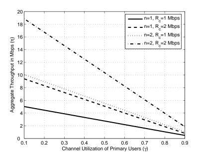
Fig. 27. The aggregate throughput against the channel utilization of PUs, when the number (M) of licensed channels is set to be 30, the number (u) of contending SUs is set to be 30, and  $CW_{min} = 256$ .
