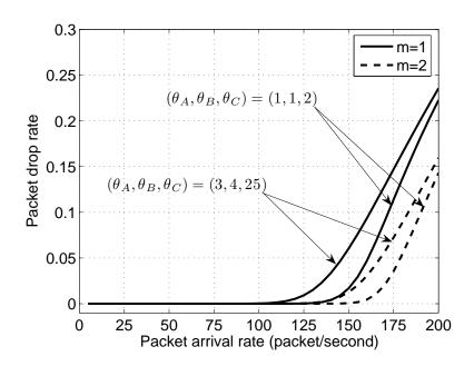
Fig. 51. The packet drop rate against the packet arrival rate. The average SNR  $(\overline{\gamma})$  is 10 dB.
