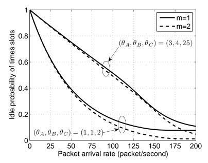
Fig. 47. The idle probability of time slots against the packet arrival rate. The average SNR ( $\overline{\gamma}$ ) is 10 dB.
