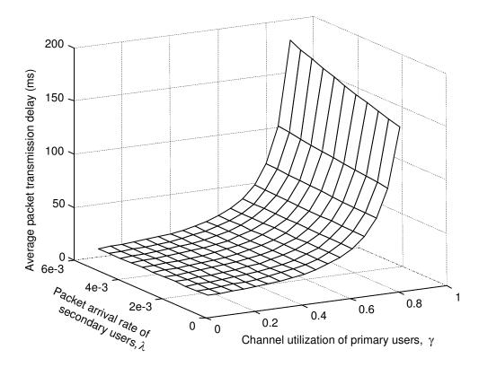
Fig. 13. The average packet transmission delay  $(W_s)$  varies with different  $\gamma$ 's and  $\lambda$ 's under negotiation-based sensing policy. The number (n) of licensed channels is 5 and the number (u) of SUs is 20.
