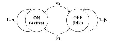
Fig. 3. The ON-OFF channel usage model for PUs.
