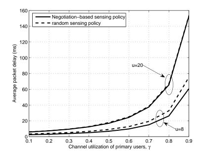
Fig. 11. The average packet transmission delay  $(W_s)$  against the channel utilization  $(\gamma)$  of PUs with different number of SUs (u) when the system utilization  $(\rho)$  of SUs is 0.1. The number (n) of licensed channels is 5. The solid lines represent the negotiation-based sensing policy, and the dashed lines represent the random sensing policy.
