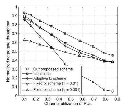
Fig. 40. The normalized aggregate throughput vs. channel utilization of PUs when the PUs' activity follows the gamma distribution.
