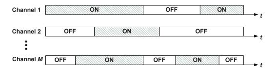
Fig. 21. Illustration of PUs' channel utilization in cognitive-radio based DSA networks. There are *M* licensed channels. The ON and OFF states of PUs operating at different licensed channels are unsynchronized.
