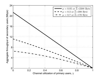
Fig. 18. The aggregate throughput of SUs against the channel utilization of PUs. The packet generation rate  $\lambda = 0.5$ . The number of SUs N = 20. The average packet size is set to 2388, 398 and 170 bytes, respectively.
