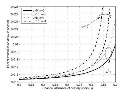
Fig. 29. The packet transmission delay against the channel utilization of PUs with the combinations of the number (u) of contending SUs being set to be 5 or 10 and the number (n) of licensed channels being set to be 4 or 5.
