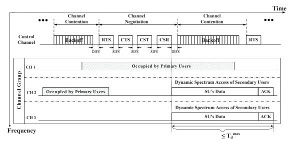
Fig. 23. Illustrations of the CREAM-MAC protocol for an example case with 1 control channel and 3 data channels (CH 1, CH 2, CH 3) which form a Channel Group.
