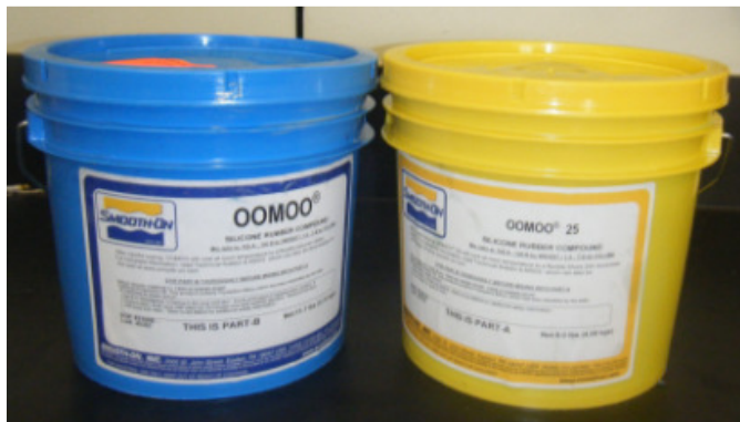
Fig. 26. Silicone rubber used for dielectric SIFA fabrication
