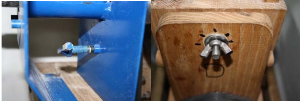
Fig. 3. Burr gap control screw: Ewing III mill (left), Omega VI mill (right).
