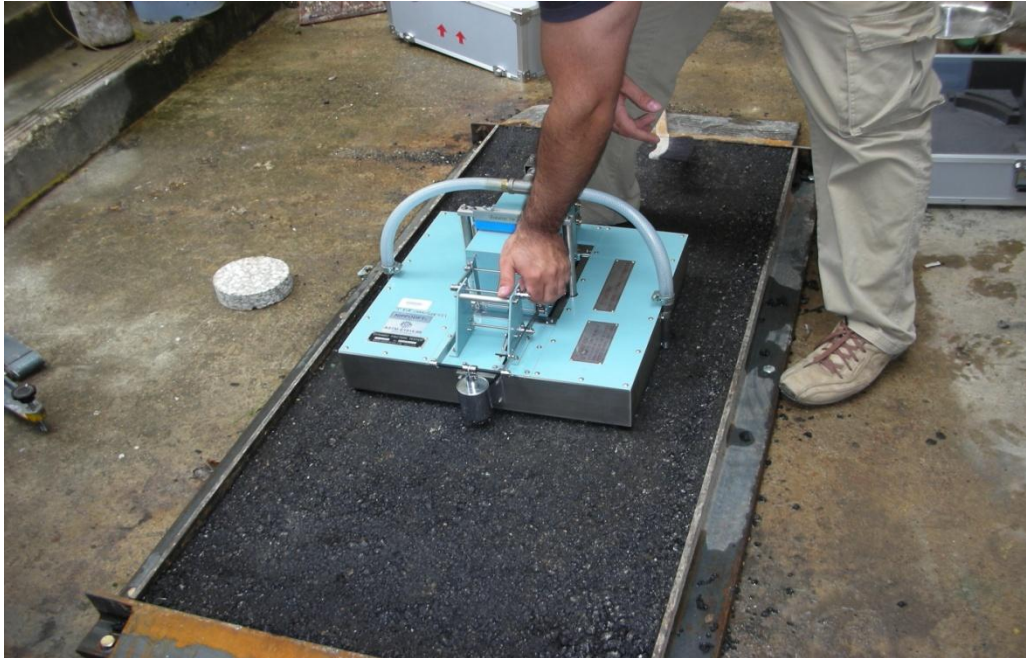
FIGURE 42 Schematic of measuring pavement skid resistance by DFT.
