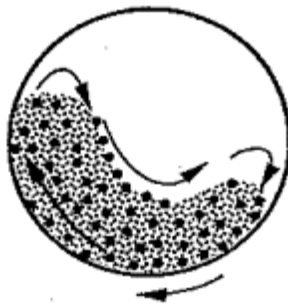
FIGURE 32 Mechanism of aggregate and steel ball interaction in Micro-Deval apparatus.
