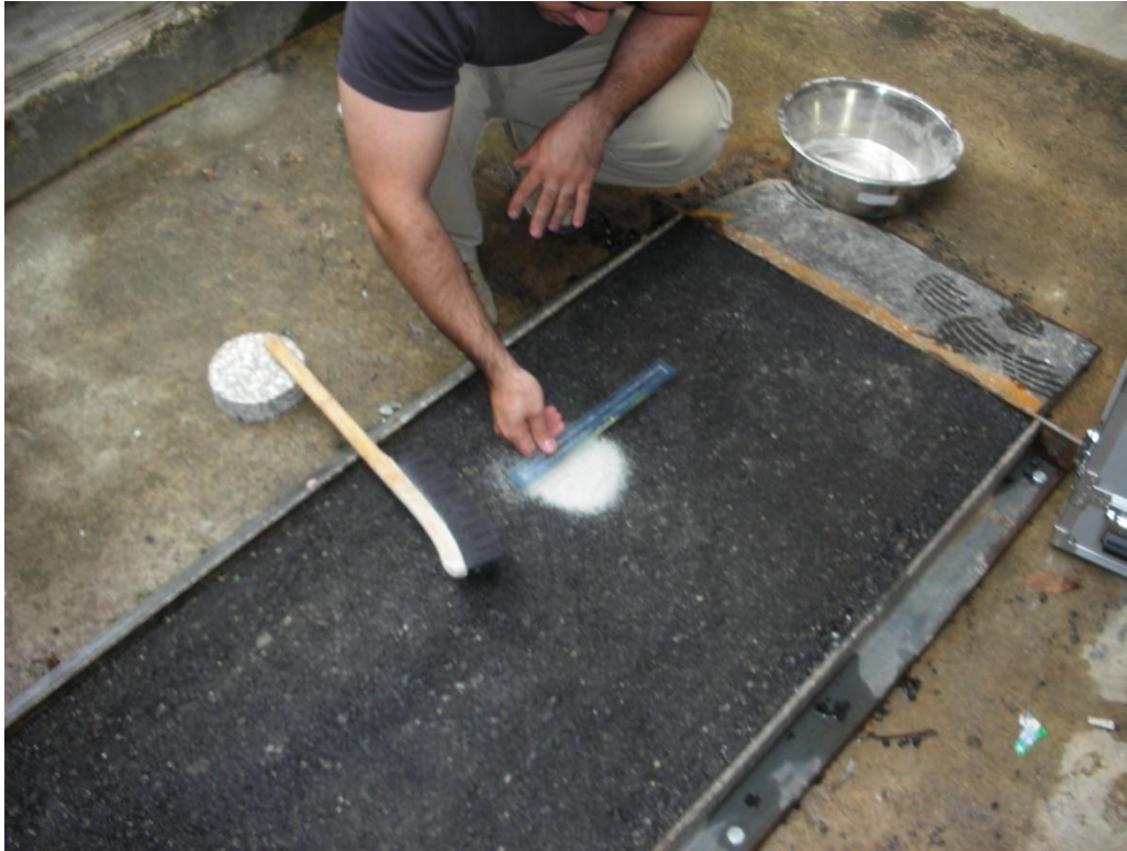
FIGURE 41 Schematic of sand patch method.
