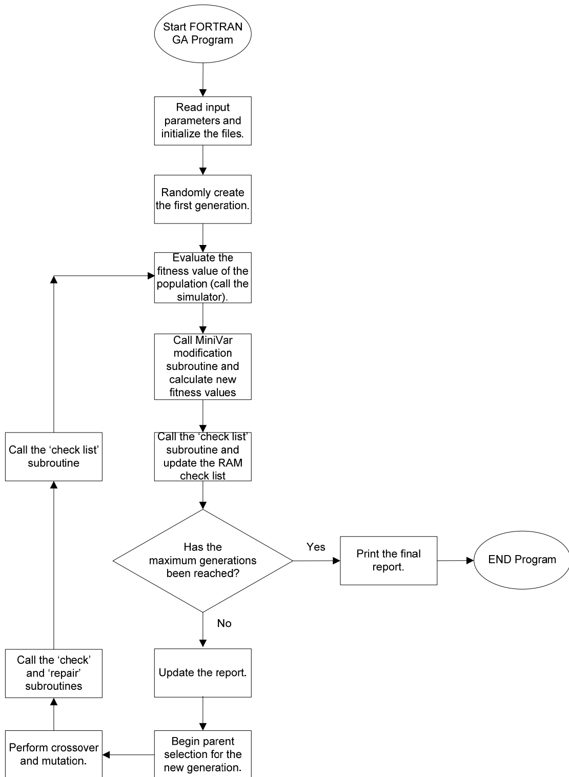
Figure 3.7 – Modified Genetic Algorithm Program Flow Chart, Without Probability of Success.
