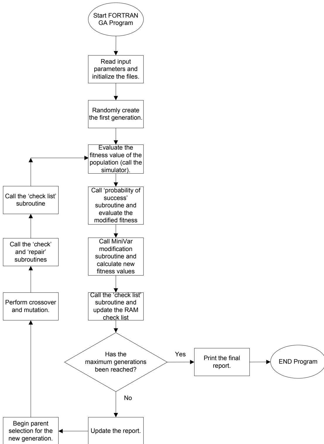
Figure 3.16 – Modified Genetic Algorithm Program Flow Chart.
