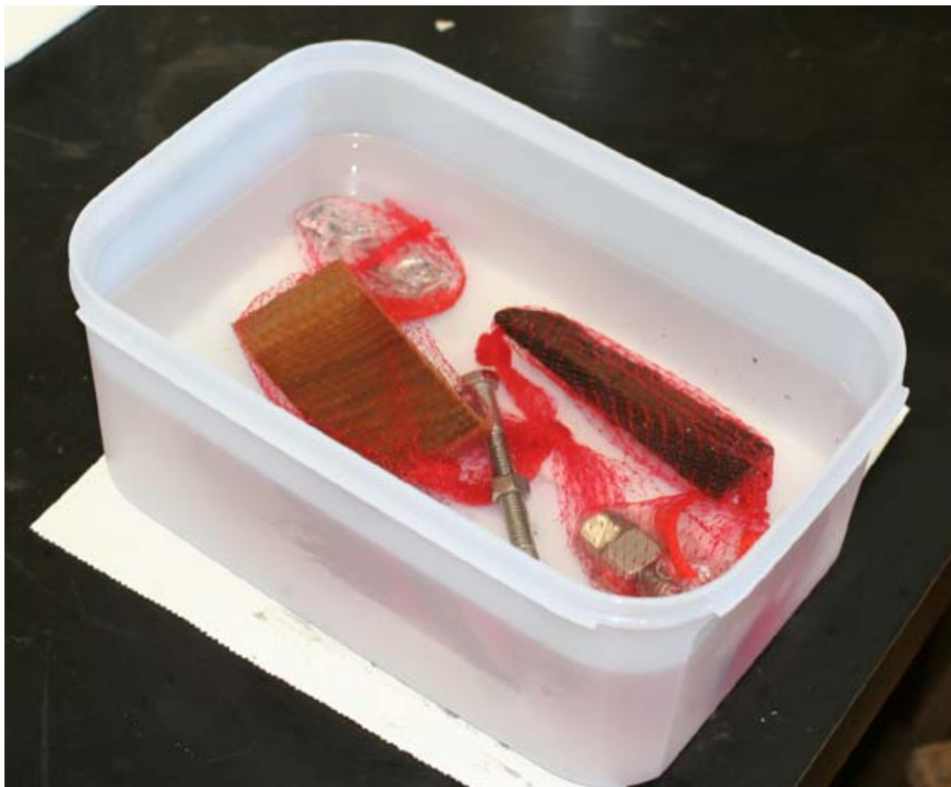
Figure 43. Container with the polymer mixture. Several sub-samples immersed into the polymer solution with the assistance of a plastic net and some improvised weights (bolts and nuts).
