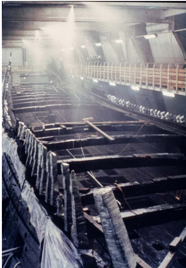
Figure 7. The Vasa being conserved through the automatic spraying system (Courtesy Archives, the Swedish National Maritime Museums).
