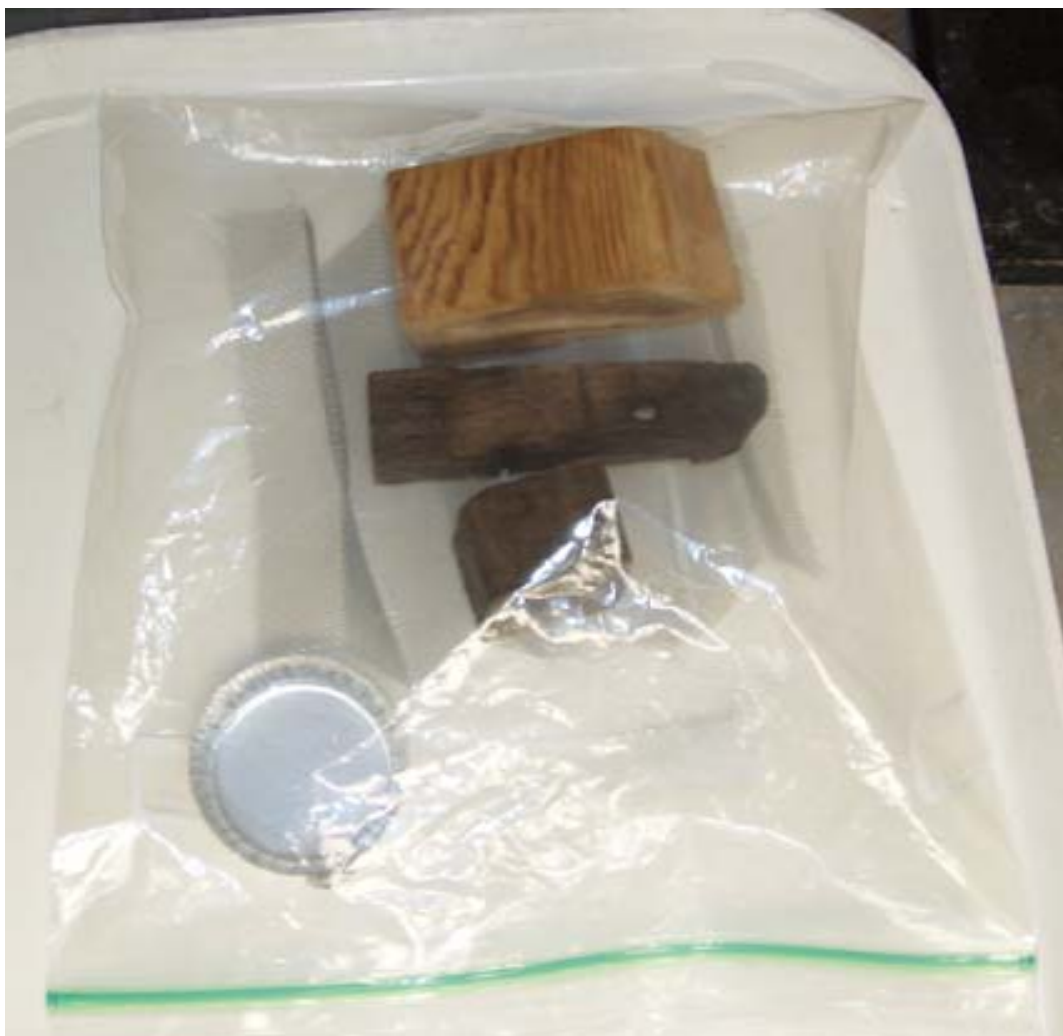
Figure 44. Catalysis of the samples. Three sub-samples during catalysis through vapor deposition inside a sealed plastic bag.
