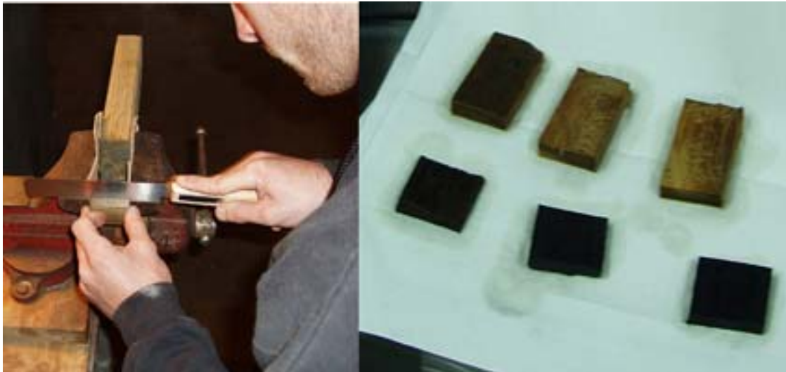
Figure 20. Two images of the slicing process. Left, Christopher Atkinson slicing one of the sub-samples with a Japanese saw; right, the resulting slices of EDMA sub-sample (three on top) and waterlogged sub-sample (three on the bottom).
