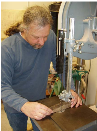
Figure 16. Wood samples being divided. Glen Grieco using a band saw for dividing the samples.
