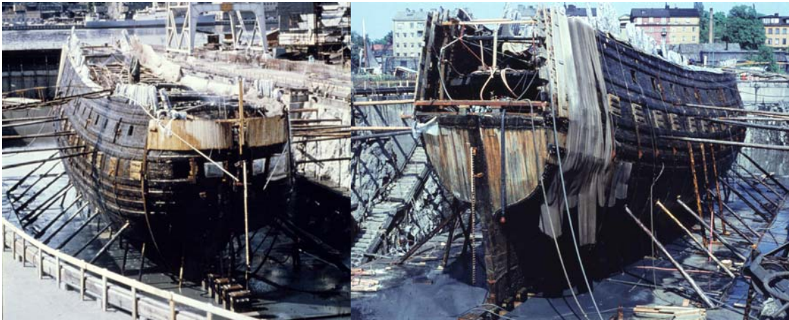
Figure 3. The Vasa hull reinforced on the floating pontoon in the dry dock (Courtesy Archives, the Swedish National Maritime Museums).
