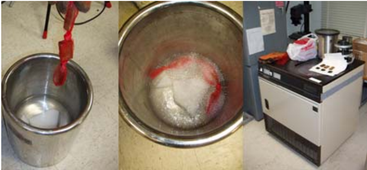
Figure 23. Three images of the freeze drying process. Left and center, samples are flash frozen in acetone and dry ice; right, the CRL freeze dryer used to dry the samples.
