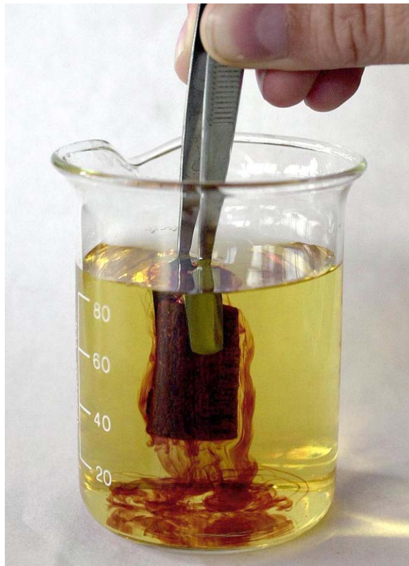
Figure 11. Aqueous solution of EDMA. Iron corrosion products being extracted from a wood sample in an EDMA solution (Courtesy Archives, the Swedish National Maritime Museums. Photographer, Stefan Evensen).
