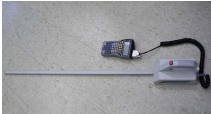
Figure 2.3. SunScan canopy analyzer.
