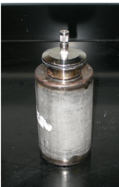
Figure 3-3. Photograph of the stainless-steel fermentor (clamp not shown).
