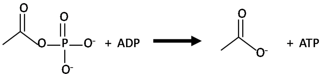
Figure T-15. Conversion of acetyl-phosphate to acetate.
