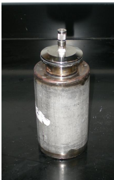
Figure 2-5. Photograph of the stainless-steel fermentor (clamp removed).
