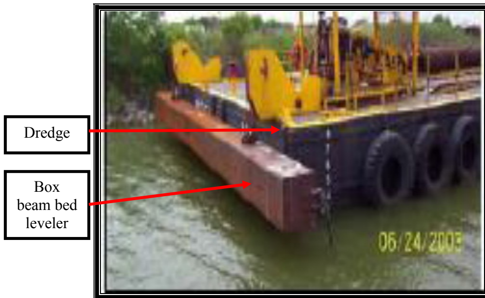
Figure 1. Box beam bed leveler attached to a dredge (courtesy of Weeks Marine).
