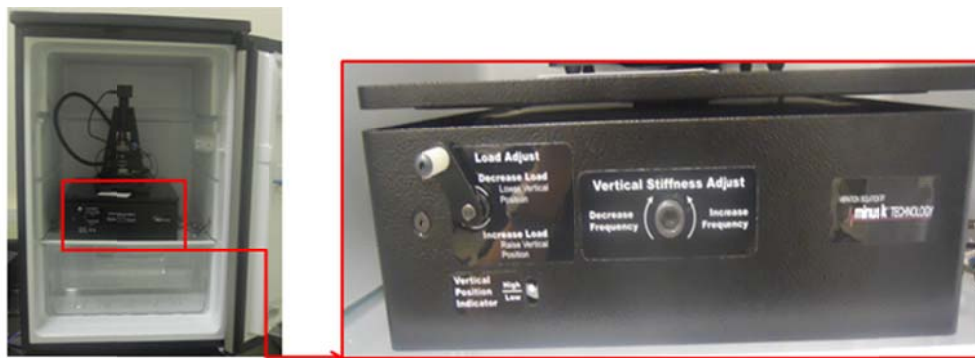
Figure 3.3. AFM environmental enclosure and floating vibration isolation stage.
