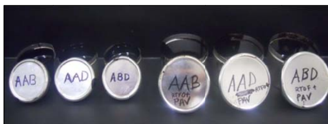
Figure 3.5. Original and aged asphalts AAB, AAD and ABD.
