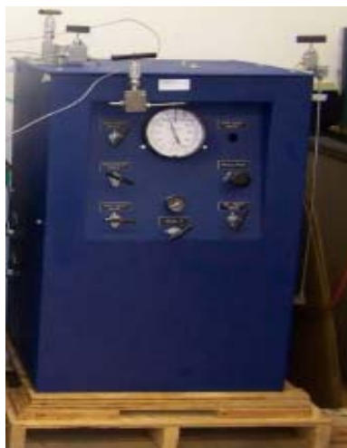
Figure 4-3. Gas booster system used to compress gas in this study
