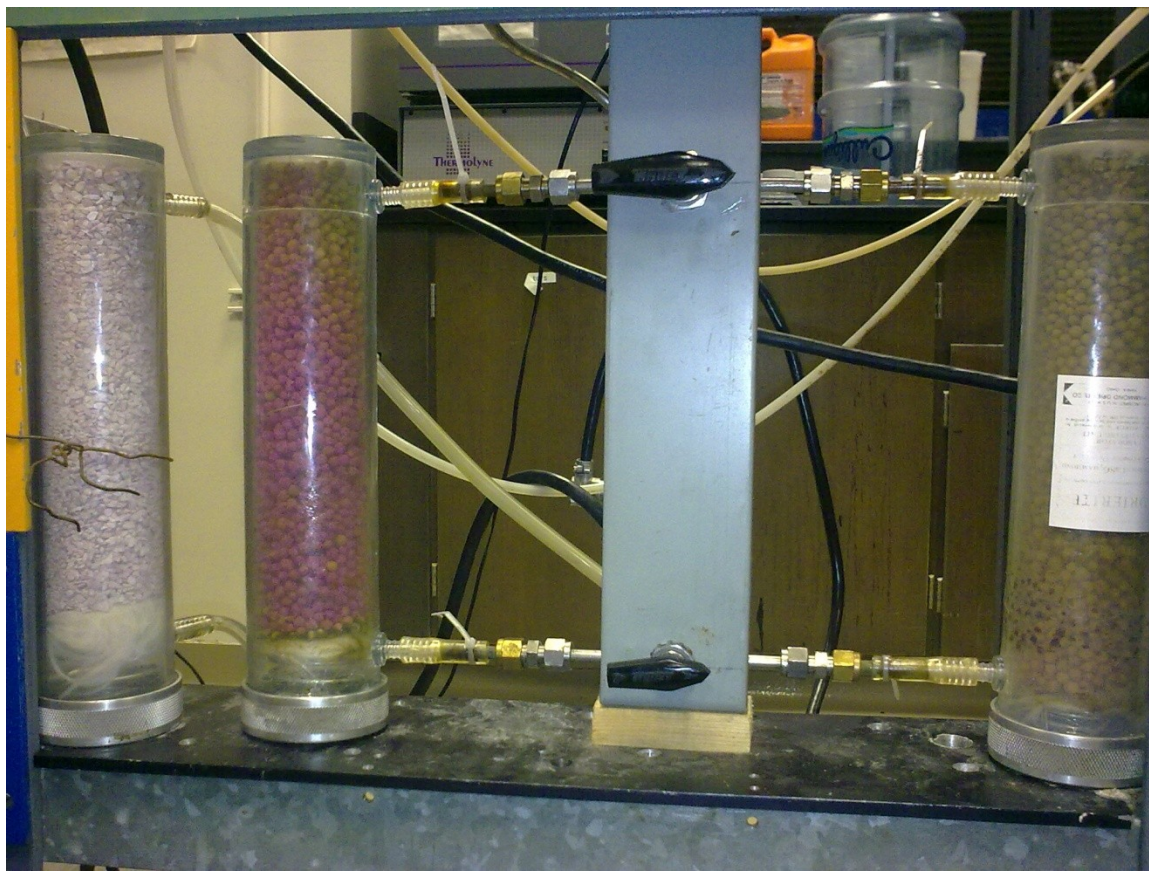
Fig. 3.9 – Acid scrubber and drierite columns.
