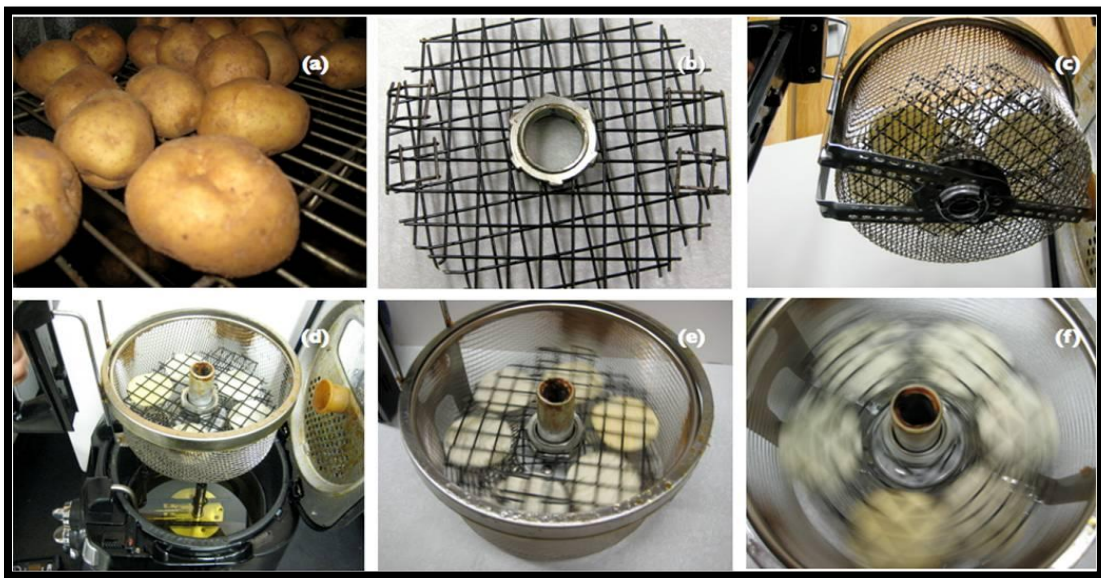
Figure 3.2: (a) Raw potato used for frying; (b) slices holding net; (c) basket with potato slices; (d) basket being placed inside the fryer; (e) potato slices being de-oiled; (f) high speed centrifuge de-oiling the chips.
