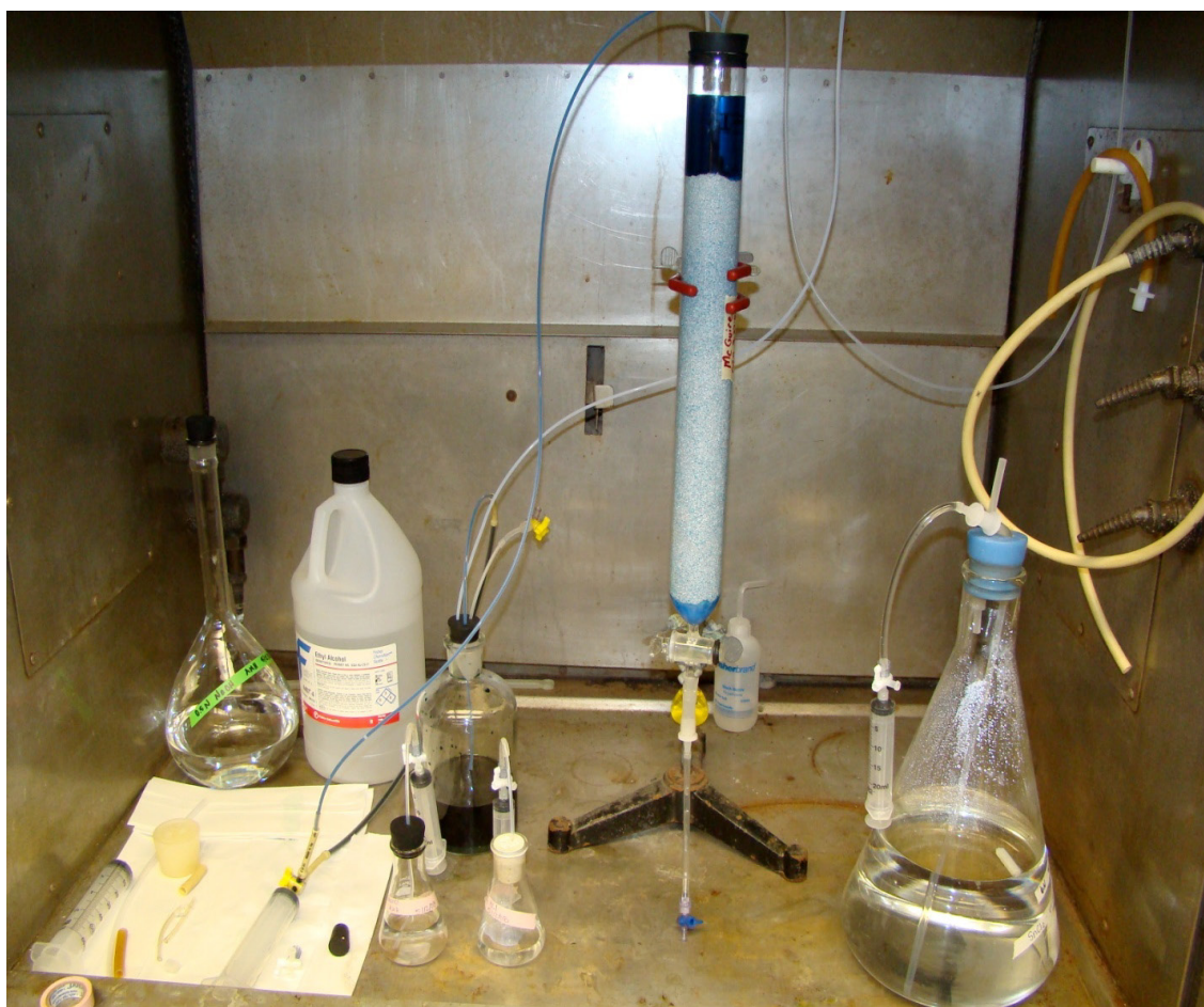
Figure 5. Photograph showing the Jones Reductor Column with \text{CrCl}_3 undergoing reduction (turning from a shade of dark forest green to the bright blue as seen above).
