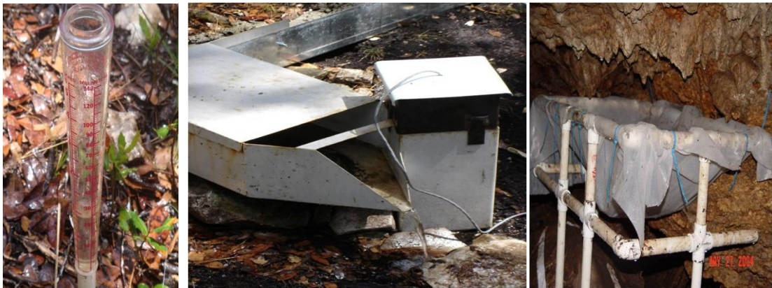
Figure 4: Picture of rain gauge used to collect throughfall (left). Picture of H-flume used to measure surface runoff (center). Picture of drip collector used to collect and measure cave recharge (right). Water collected was piped to a tipping bucket for quantity (liters) measurement.
