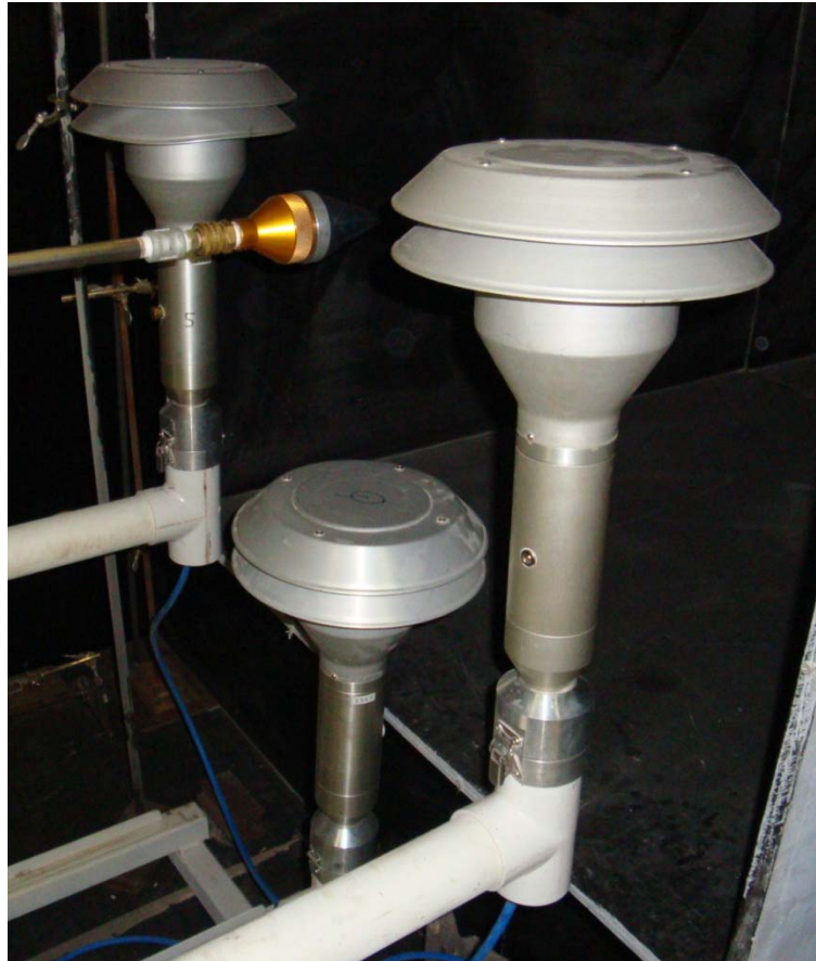
Figure 8. Photograph of the test chamber with the isokinetic and PM 10 sampler inlets.
